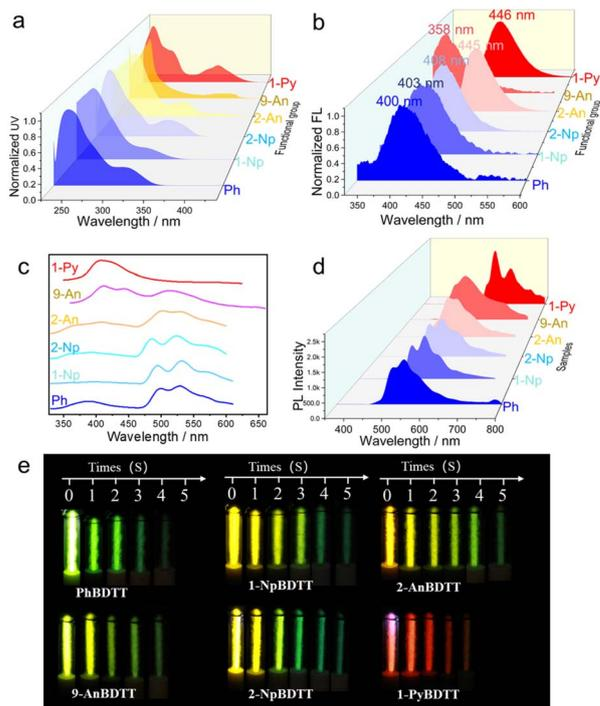
Fig. 2 a) Absorption spectra and (b) PL spectra of **BDTT-Ars** in DCM,  $[\text{C}] = 1.0 \times 10^{-5}$  M. (c) Steady state photoluminescence spectra and (d) delayed emission spectra of **BDTT-Ars** in 2-MTHF ( $[\text{C}] = 1.0 \times 10^{-5}$  M) at 77 K (0.5 ms, delayed). (e) Long afterglow photographs of **BDTT-Ars** in 2-MTHF in quartz tubes at 77 K under irradiation of a 365 nm lamp (5 W).
