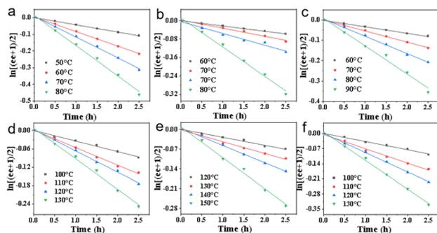
Fig. 3 Kinetic measurements of the racemization of BD TT-Ars (a–f: BD TT-Ph, BD TT-1Np, BD TT-2Np, BD TT-2An, BD TT-9An and BD TT-1Py, respectively).
