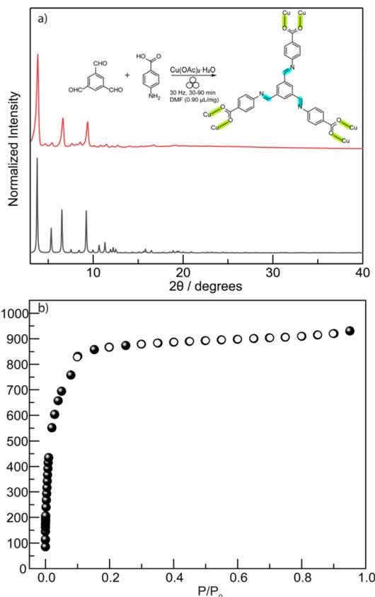
Fig. 5 (a) The PXRD pattern of mechanochemically obtained solids derived from the imine-linked ligand (red line) is compared to the calculated pattern from the amide-linked **pto**-topology MOF (black line). (b) N<sub>2</sub> adsorption isotherms at 77 K were collected for the imine-based **pto**-topology MOF prepared mechanochemically.
