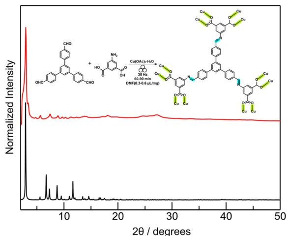
Fig. 4 An expanded **rht**-topology MOF featuring the imine-linkage allows for mechanochemical synthesis, confirmed by PXRD patterns (red line, as-synthesized; black line, calculated from the amide-linked isostructural MOF).
