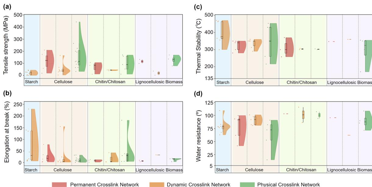
**Scheme 4** Representative material properties of permanent, dynamic, and physical crosslinked bioplastic networks across various biopolymers and raw biomass. (a) Tensile strength; (b) elongation at break; (c) thermal stability; (d) water resistance.
