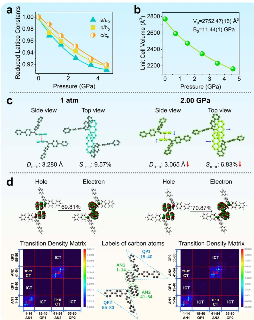
Fig. 3 (a) Compression ratios of the crystallographic axes and (b) evolution of unit cell volume of QP-AN crystals under pressure ( $V_0$  and  $B_0$  denote the volume and the bulk modulus of elasticity under ambient pressure). (c) Dimeric geometry and (d) calculated NTOs and TDM maps of QP-AN crystals at 1 atm and 2.00 GPa. Carbon atoms are numbered sequentially by fragment for TDM analysis, and hydrogen atoms are omitted due to their negligible contribution to the transitions of interest.
