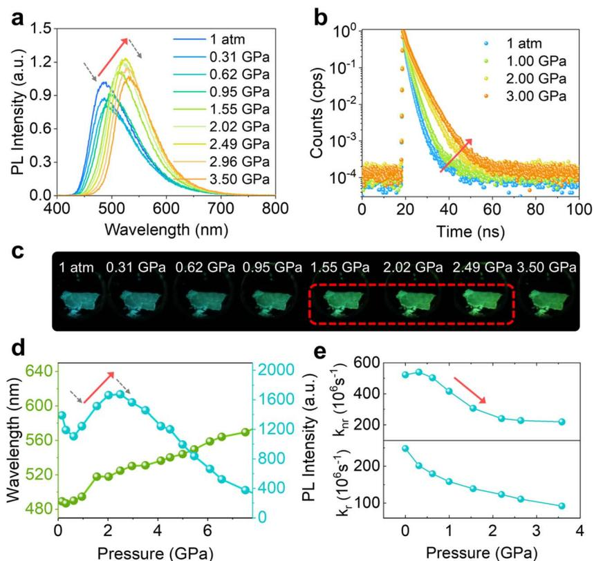
Fig. 2 (a) *In situ* high-pressure PL spectra and (b) time-resolved PL spectra of QP-AN crystals at various pressures from 1 atm to 3.50 GPa. (c) Corresponding fluorescence photographs of QP-AN crystals under pressures ranging from 1 atm to 3.50 GPa. (d) Pressure-dependent plots of maximum emission wavelength and PL intensity. (e) Pressure-dependent  $k_r$  and  $k_{nr}$  of QP-AN crystals.
