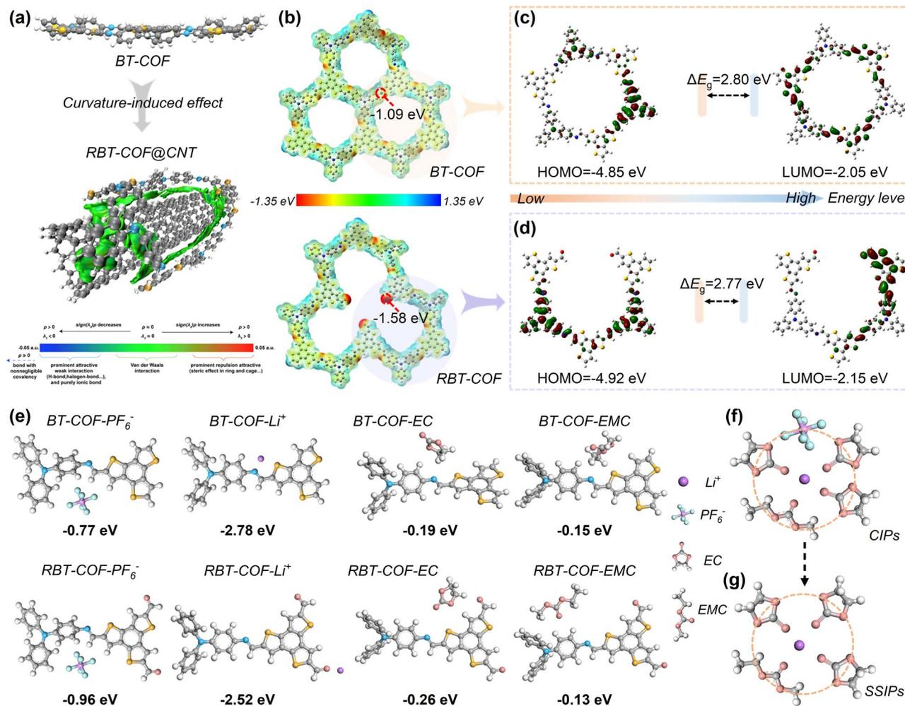
Fig. 2 (a) A representation of the structural change from BT-COF to RBT-COF@CNT and weak interaction regions visualized with a  $\delta_g^{\text{inter}}$  isovalue of 0.005 a.u. in the IGMH analysis for RBT-COF@CNT. (b) MESP of BT-COF and RBT-COF. The HOMO and LUMO energy levels with the energy gap of the structural units for (c) BT-COF and (d) RBT-COF. (e) The binding energies of BT-COF and RBT-COF with different electrolyte compositions. The solvation structure in (f) BT-COF and (g) RBT-COF.
