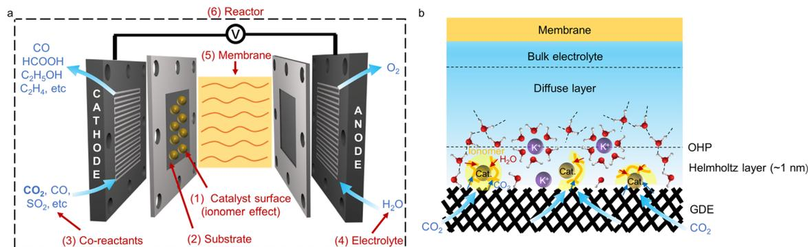
Fig. 2 (a) Influencing factors on the microenvironment in the electrocatalytic CO<sub>2</sub>RR. (b) Schematic illustration of the microenvironment at the catalyst surface modulated by ionomers. The terms Cat. and OHP represent the catalyst and Outer Helmholtz Plane, respectively.
