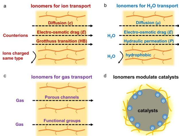
Fig. 3 Functional mechanisms of ionomers transferring (a) ions, (b) H<sub>2</sub>O, (c) gas, and (d) modulating catalysts (where  $c$ ,  $E$ ,  $HB$ ,  $\mu$ ,  $P$ , and  $e$  represent the concentration, potential, hydrogen bond, chemical potential, pressure, and electron, respectively).
