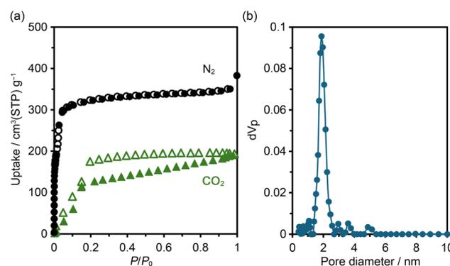
Fig. 4 (a) Gas sorption isotherms for  $\text{N}_2$  at 77 K (black) and  $\text{CO}_2$  at 195 K (green). (b) Pore width distribution using the NLDFT model for the  $\text{N}_2$  adsorption isotherm.
