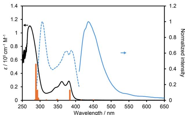
Fig. 5 Absorption (black solid line), fluorescence (cyan solid line), and excitation (cyan dotted line) spectra of **NDITA** in DMF solution. Calculated one-electron transition oscillations are shown with orange bars in arbitrary units. The fluorescence spectrum was measured at the excitation wavelength of 381 nm. The excitation spectrum was recorded at 430 nm.
