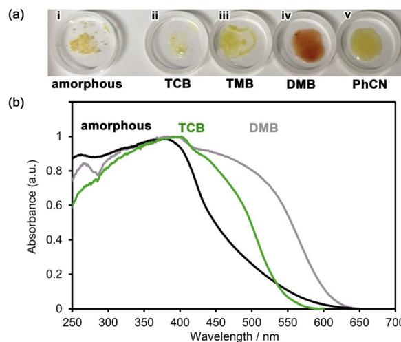
Fig. 6 (a) Photographs of solvent-immersed bulk crystals of the HOF **NDITA-1**: (i) amorphous solid, (ii) as-formed **NDITA-1(TCB)**, (iii) TMB-immersed HOF, (iv) DMB-immersed HOF and (v) PhCN-immersed HOF. (b) Normalized diffuse reflectance spectra of the amorphous solid (black), **NDITA-1(TCB)** (green) and DMB-immersed HOF (grey). The spectra were adjusted to zero at 650 nm.
