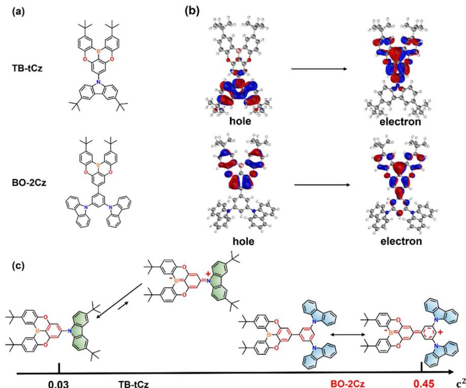
Fig. 2 (a) The structures of TB-tCz and BO-2Cz; (b) the NTOs of TB-tCz and BO-2Cz; (c) the  $c^2$  value and the resonance structures of TB-tCz and BO-2Cz.
