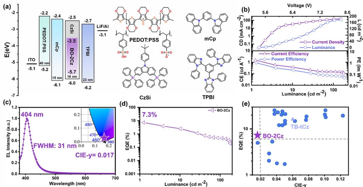
Fig. 5 (a) The energy level diagram and the structures of functional layer materials in the OLED; (b) the current density–voltage–luminance ( $J$ – $V$ – $L$ ) and the current efficiency–luminance–power efficiency (CE–L–PE) curves of BO-2Cz; (c) the normalized electroluminescence spectra and the CIE coordinates of BO-2Cz OLED; (d) The efficiency–luminance (EQE–L) curve of BO-2Cz; (e) The comparison of the device properties between BO-2Cz and the devices that have been reported.
