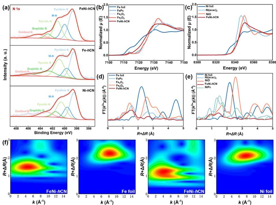
Fig. 2 (a) High-resolution XPS spectra of N 1s for the FeNi-hCN, Fe-hCN and Ni-hCN catalysts. (b) Fe K-edge XANES spectra. (c) Ni K-edge XANES spectra. (d) Fe K-edge  $k^3$ -weighted Fourier Transform (FT) EXAFS spectra. (e) Ni K-edge  $k^3$ -FT-EXAFS spectra. (f) WT EXAFS contour plots of Fe K-edge for FeNi-hCN and Fe foil, Ni K-edge for FeNi-hCN, and Ni foil.
