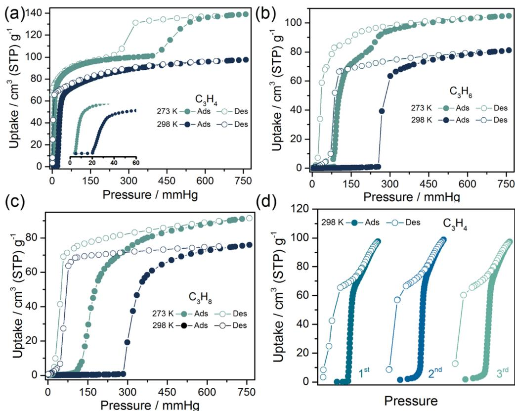
Fig. 2 The sorption isotherms recorded at 273 K and 298 K for (a)  $C_3H_4$ , (b)  $C_3H_6$  and (c)  $C_3H_8$ . The inset in (a) highlights the low gate-opening pressures. (d) Three cycles of  $C_3H_4$  sorption isotherms at 298 K.
