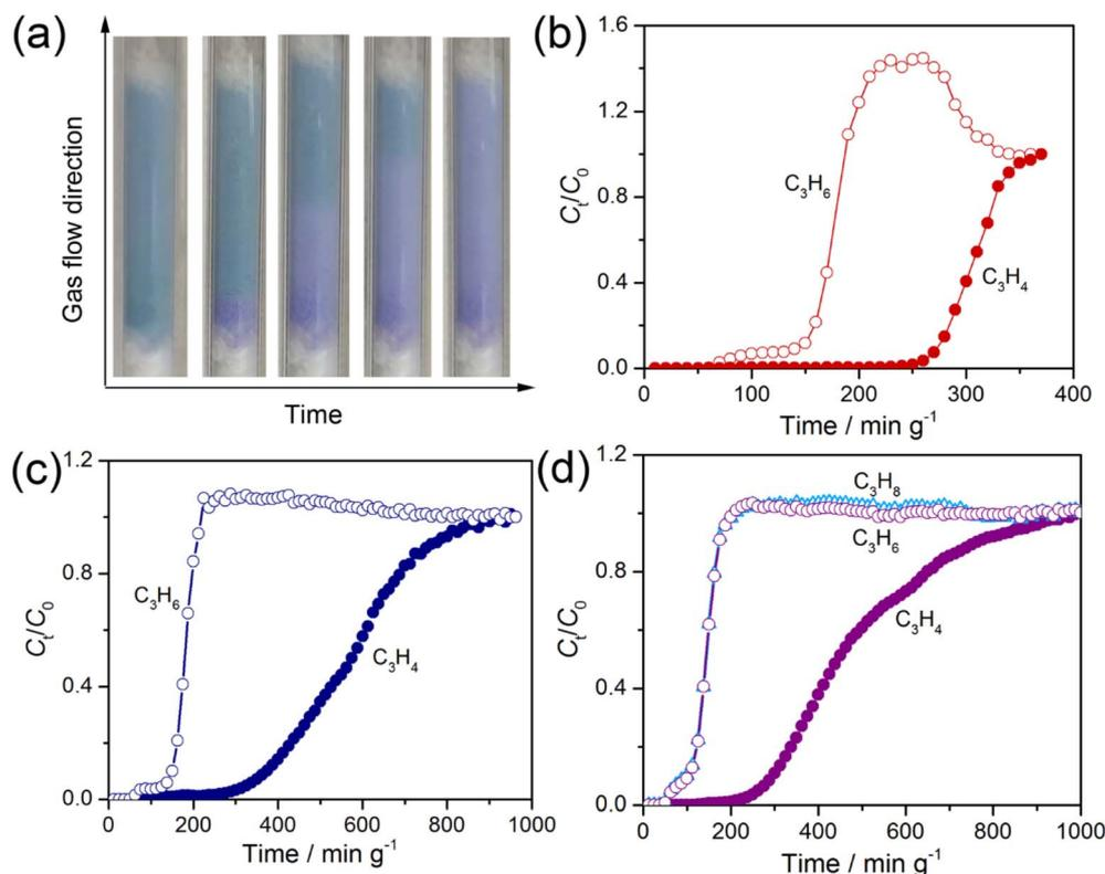
Fig. 6 (a) Sample was packed in the column and underwent a colour change along the gas flow direction over time. (b–d) Experimental breakthrough curves for 40/60 (v/v) and 10/90 (v/v) C<sub>3</sub>H<sub>4</sub>/C<sub>3</sub>H<sub>6</sub> binary mixtures (b and c) and a 10/40/50 (v/v/v) C<sub>3</sub>H<sub>4</sub>/C<sub>3</sub>H<sub>6</sub>/C<sub>3</sub>H<sub>8</sub> ternary mixture (d).
