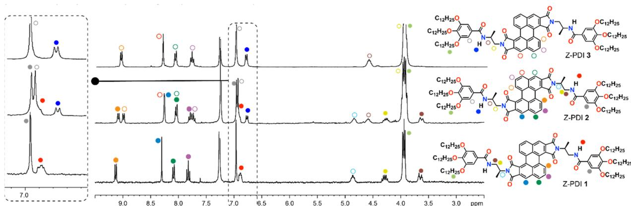
Fig. 2 Partial  $^1\text{H}$  NMR spectra of Z-PDIs 1–3 showing the aromatic and part of the aliphatic protons. The left part of the panel depicts the zoomed in region of the amide protons (experimental conditions:  $\text{CDCl}_3$ ; 298 K; 300 MHz).
