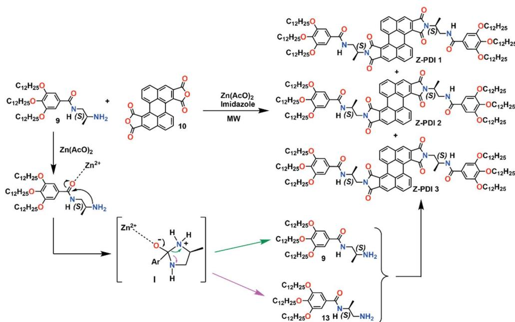
Scheme 1 Proposed Zn<sup>2+</sup>-catalyzed intramolecular transamidation mechanism yielding a mixture of the three isomeric Z-PDIs 1–3.
