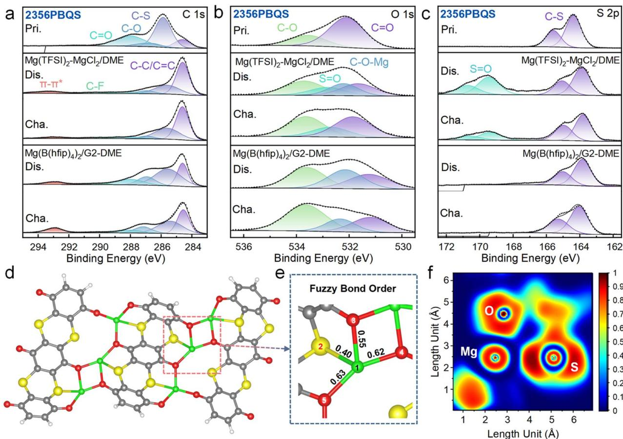
Fig. 5 (a) C 1s, (b) O 1s, and (c) S 2p XPS spectra of 2356PBQS in the pristine and charge/discharge states in Mg(TFSI)<sub>2</sub>-MgCl<sub>2</sub>/DME and Mg(B(hfip)<sub>4</sub>)<sub>2</sub>/G2-DME electrolytes. (d) Molecular structure, (e) partial view with fuzzy bond orders and (f) ELF of 2356PBQS–Mg (Mg1, S2 and O5).
