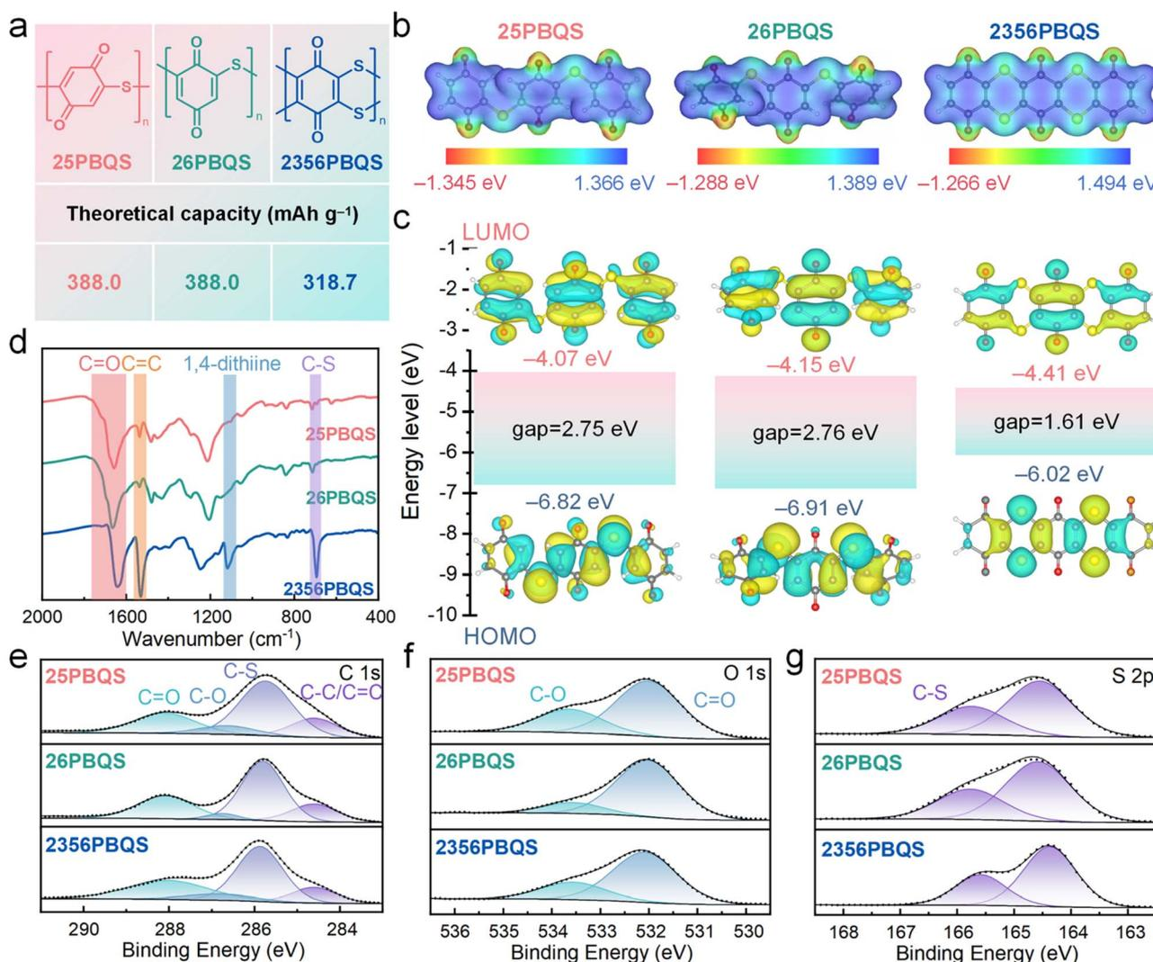
Fig. 1 (a) Structures and theoretical capacities, (b) ESP surfaces, (c) HOMO–LUMO energy level diagrams, (d) FTIR spectra, and (e) C 1s, (f) O 1s and (g) S 2p XPS spectra of 25PBQS, 26PBQS and 2356PBQS.
