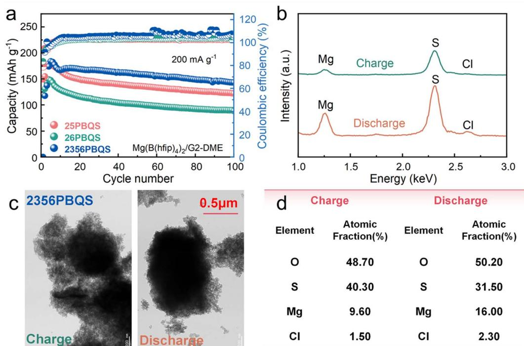
Fig. 3 (a) Cycling performances of 25PBQS, 26PBQS and 2356PBQS in Cl-free Mg(B(hfip))<sub>4</sub>/G2-DME electrolyte. (b) EDS spectra, (c) TEM images and (d) elemental compositions of 2356PBQS at the charge/discharge states of the 35th cycle in Cl-containing Mg(TFSI)<sub>2</sub>-MgCl<sub>2</sub>/DME electrolyte.
