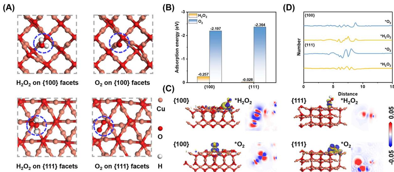
Fig. 5 (A) Optimized adsorption models for different adsorbates on the {100} and {111} facets of Cu<sub>2</sub>O. (B) Adsorption energy diagram of different adsorbates on {100} and {111} facets. (C) Differential charge density analysis of different adsorbates on {100} and {111} adsorption models. (D) The variation of electron transfer number along the *c*-axis of the cell as a function of distance.
