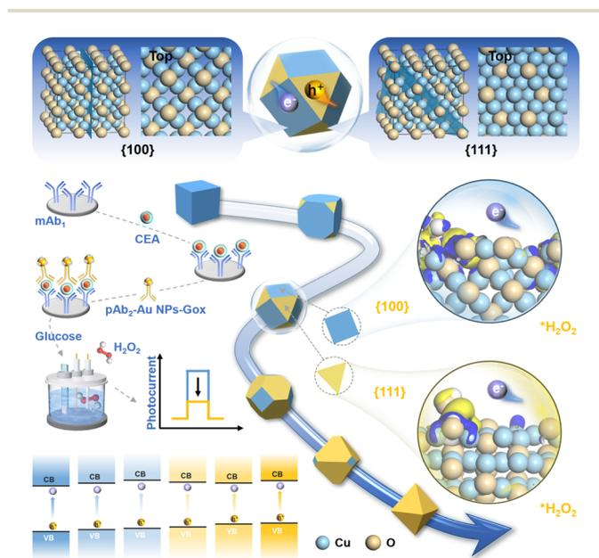
**Scheme 1** Schematic illustration of tuning the anisotropic facet of Cu<sub>2</sub>O single-crystals for photocarrier spatial segregation-based photoelectrochemical immunoassay.
