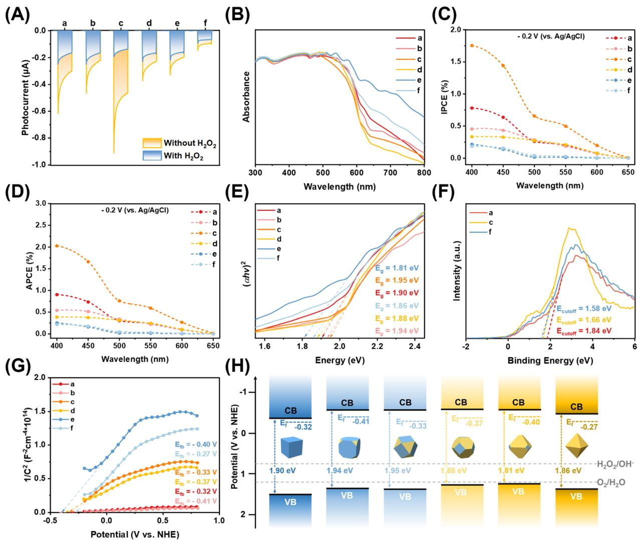
Fig. 3 (A) Photoelectric response curves, (B) UV-vis diffuse reflectance spectra, (C) IPCE plot, (D) APCE plot, (E) bandgap width spectra, (F) XPS-VB spectra, and (G) Mott-Schottky plot of (a)  $c$ - $\text{Cu}_2\text{O}$ , (b)  $t_1$ - $\text{Cu}_2\text{O}$ , (c)  $t_2$ - $\text{Cu}_2\text{O}$ , (d)  $t_3$ - $\text{Cu}_2\text{O}$ , (e)  $t_4$ - $\text{Cu}_2\text{O}$ , and (f)  $o$ - $\text{Cu}_2\text{O}$ . (H) Possible sensing mechanism.
