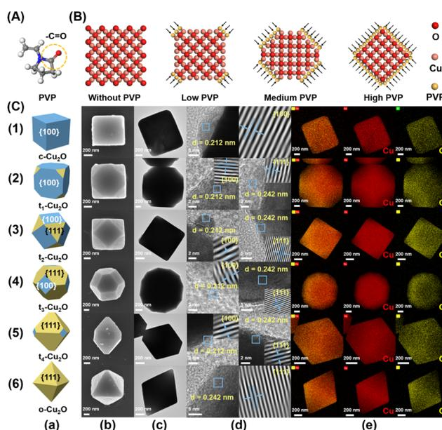
**Fig. 1** (A) Chemical structure of PVP. (B) Adsorption of PVP on the crystal facets of Cu<sub>2</sub>O. (C) (a1–a6) structural models, (b1–b6) SEM images, (c1–c6) HRTEM images, and (e1–e6) total element distribution images and single element mapping distribution of c-Cu<sub>2</sub>O, t<sub>1–4</sub>-Cu<sub>2</sub>O, and o-Cu<sub>2</sub>O.
