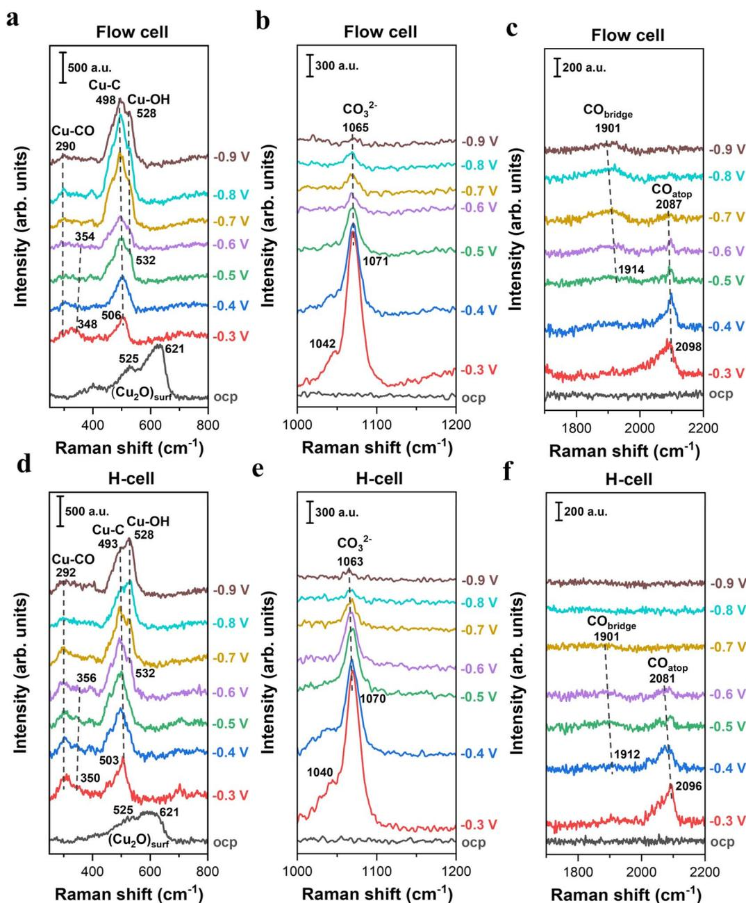
Fig. 2 *In situ* Raman spectroscopy of electrochemical CO<sub>2</sub> reduction on Cu catalysts in 0.5 M KHCO<sub>3</sub> using two representative *in situ* Raman configurations. (a–c) Raman spectra on Cu catalysts as a function of applied potentials (*vs.* RHE, no *iR* correction) collected in the GDE-type spectroelectrochemical flow cell. (d–f) Raman spectra on Cu catalysts as a function of applied potentials (*vs.* RHE, no *iR* correction) collected in the H-type spectroelectrochemical cell.
