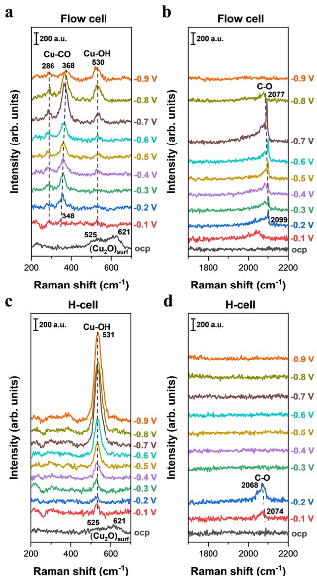
Fig. 4 *In situ* Raman spectroscopy of electrochemical CO reduction on Cu catalysts in 0.5 M KOH using two representative *in situ* Raman configurations. (a and b) Raman spectra on Cu catalysts as a function of applied potentials (vs. RHE, no *iR* correction) collected in the GDE-type spectroelectrochemical flow cell. (c and d) Raman spectra on Cu catalysts as a function of applied potentials (vs. RHE, no *iR* correction) collected in the H-type spectroelectrochemical cell.
