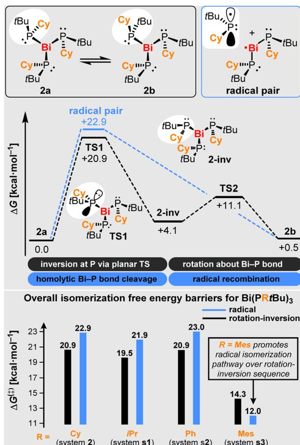
**Scheme 3** Theoretical analyses. Top: isomerization of compounds **2a** and **2b** (top left), along with mechanistic considerations proposing viable reaction pathways. Bottom: overall isomerization barriers for radical vs. rotation-inversion sequence for systems **2**, **s1**, **s2** and **s3**. Energies were determined by DFT calculations (see discussion and SI).
