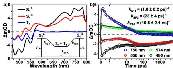
Fig. 6 Global analysis of the fsTA data of *tRc* films. (a) Species-associated spectra and kinetic model. (b) Globally fitted wavelength kinetics as well as the corresponding SF and TTA rate constants.
