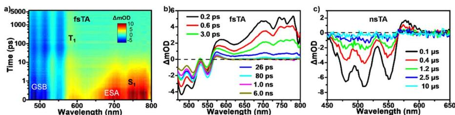
Fig. 5 SF and triplet decay processes in *tRc* thin films. (a) Pseudocolor plot and (b) selected spectra from fsTA measurements of *tRc* thin films (450 nm excitation). (c) nsTA spectra from nanosecond laser flash photolysis measurements of *tRc* thin films (532 nm-excitation,  $50 \mu\text{J cm}^{-2}$ ).
