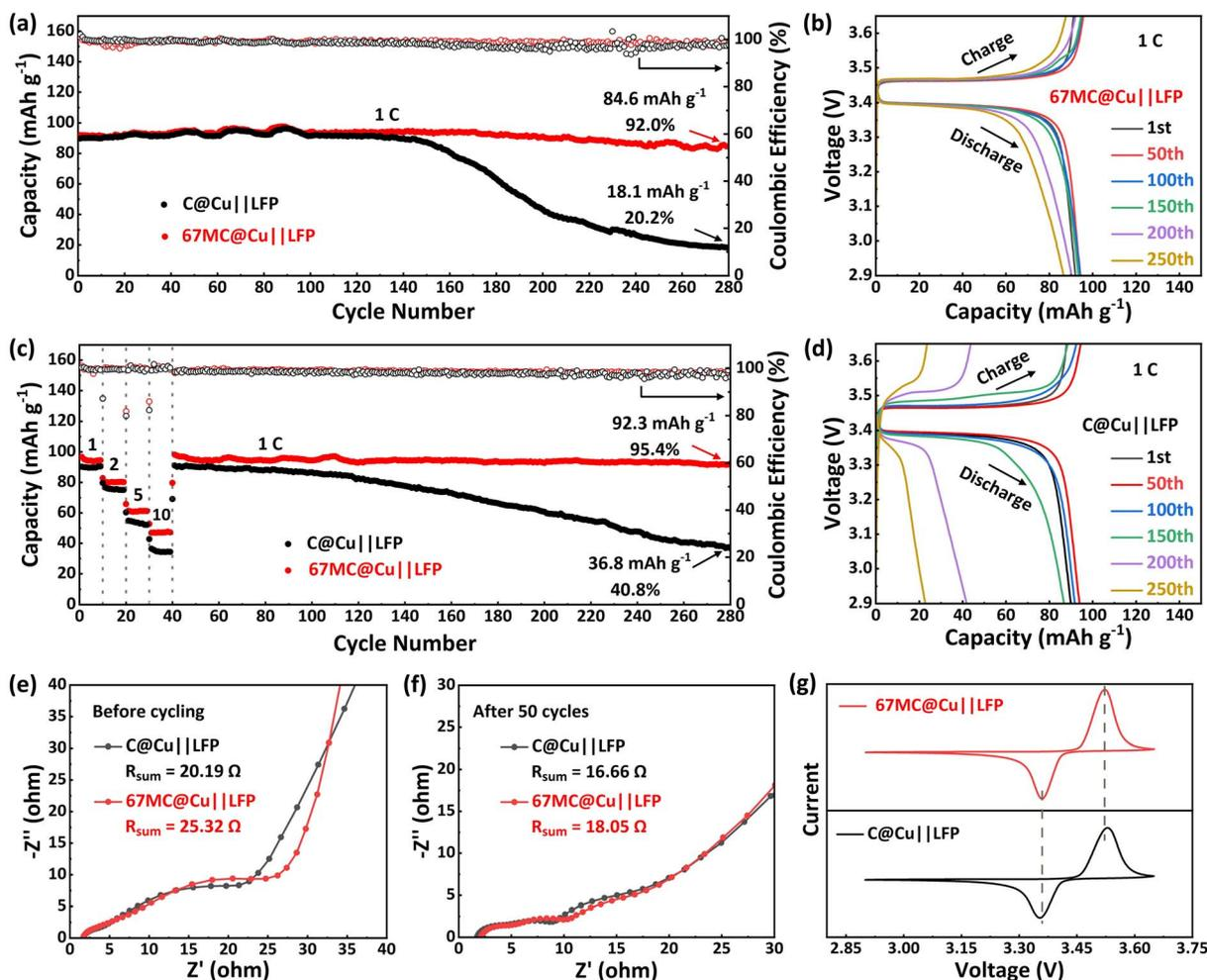
Fig. 5 (a) Cycling performance of C@Cu||LFP and 67 MC@Cu||LFP at 1C (1C = 170 mA h g<sup>-1</sup>). (prelithiation: 5 mA h cm<sup>-2</sup>; activation: 0.2C, 2 cycles). Charge and discharge curves at different cycles of (b) 67 MC@Cu||LFP and (d) C@Cu||LFP. (c) Rate performance comparison between C@Cu||LFP and 67 MC@Cu||LFP. EIS spectra of C@Cu||LFP and 67 MC@Cu||LFP (e) before cycling and (f) after 50 cycles. (g) CV curves of C@Cu||LFP and 67 MC@Cu||LFP (scan rate: 1 mV s<sup>-1</sup>).
