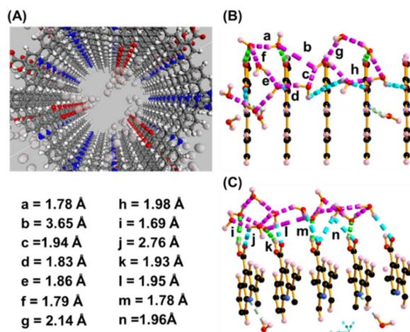
Fig. 5 CBMC simulation to understand the interaction of water with **Qy-COOH**: (A) formation of water channel in  $c$ -axis through extensive H-bonding with water molecule. (B and C) Top and sidewise view of extended H-bonded tunnels with  $-\text{COOH}$  group.
