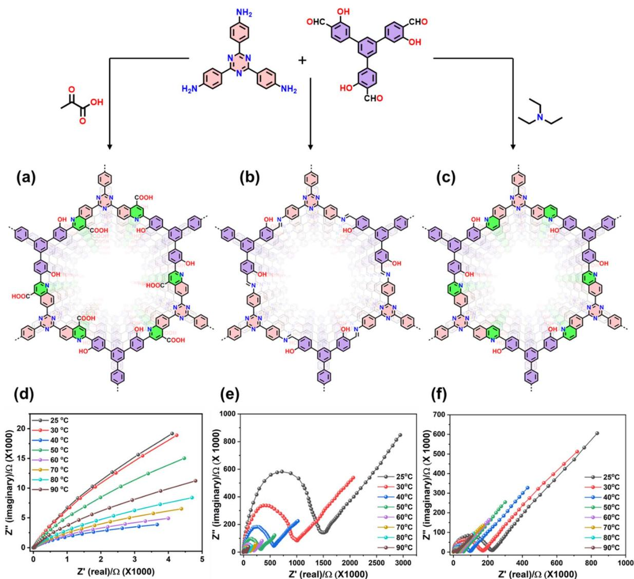
Fig. 6 Synthesis and structure of (a) **OH-Qy-COOH**, (b) **OH-Im** and (c) **OH-Qy-H**. Nyquist plots of (d) **OH-Qy-COOH**, (e) **OH-Qy-H** and (f) **OH-Im** measured under 98% RH at different temperatures showing the temperature dependence of proton conductivities.
