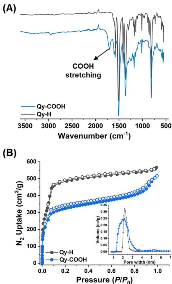
Fig. 2 (A) FTIR spectra for Qy-COOH and Qy-H; (B) N<sub>2</sub> sorption at 77 K for Qy-COOH and Qy-H; (inset) pore size distribution of Qy-COOH and Qy-H.
