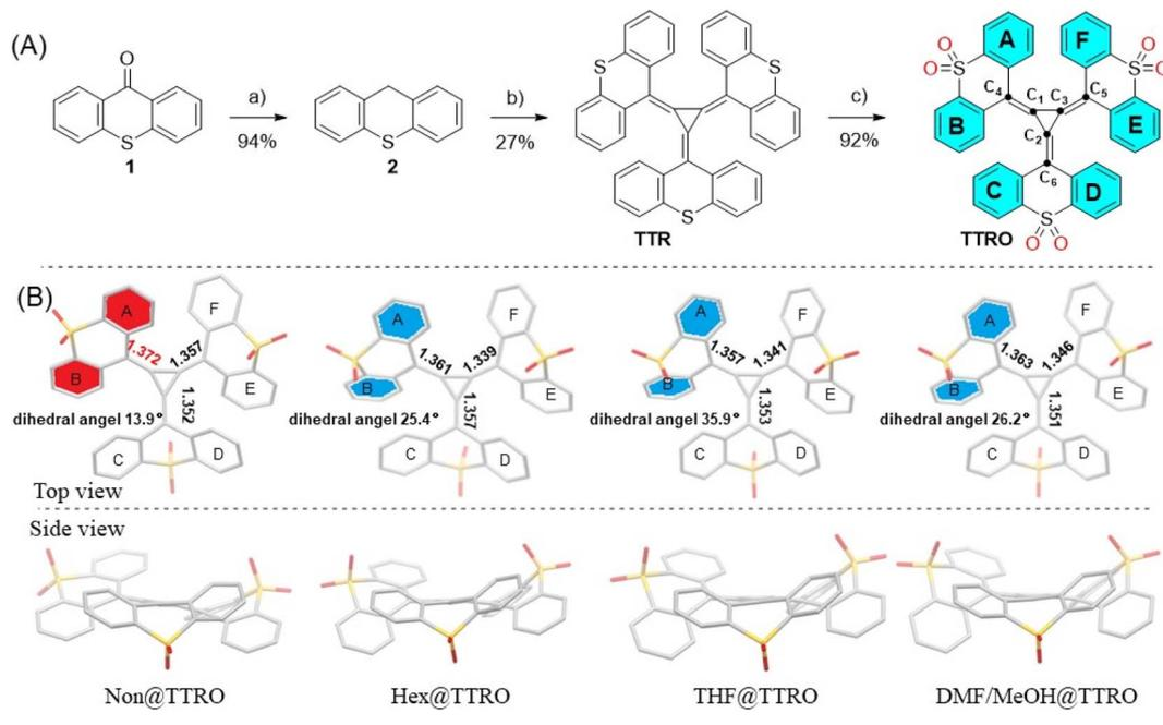
Fig. 1 (A) Synthesis of sulfone[3]radialene (TTRO). Conditions: a)  $\text{NaBH}_4$ ,  $\text{I}_2$ , THF, 0 °C to 65 °C, 12 h. b) i. *n*-BuLi, THF/DMSO (v/v = 1 : 1), 0 °C to rt, 1 h; ii. Tetrachlorocyclopropene (TCCP), 0 °C to rt, 1 h; iii. Bubbling  $\text{O}_2$ , 0 °C to rt, 1 h. c) *m*-chloroperoxybenzoic acid, DCM, rt, 12 h. (B) Crystal structures of TTRO in different crystalline frameworks with highlighted bonds and dihedral angles.
