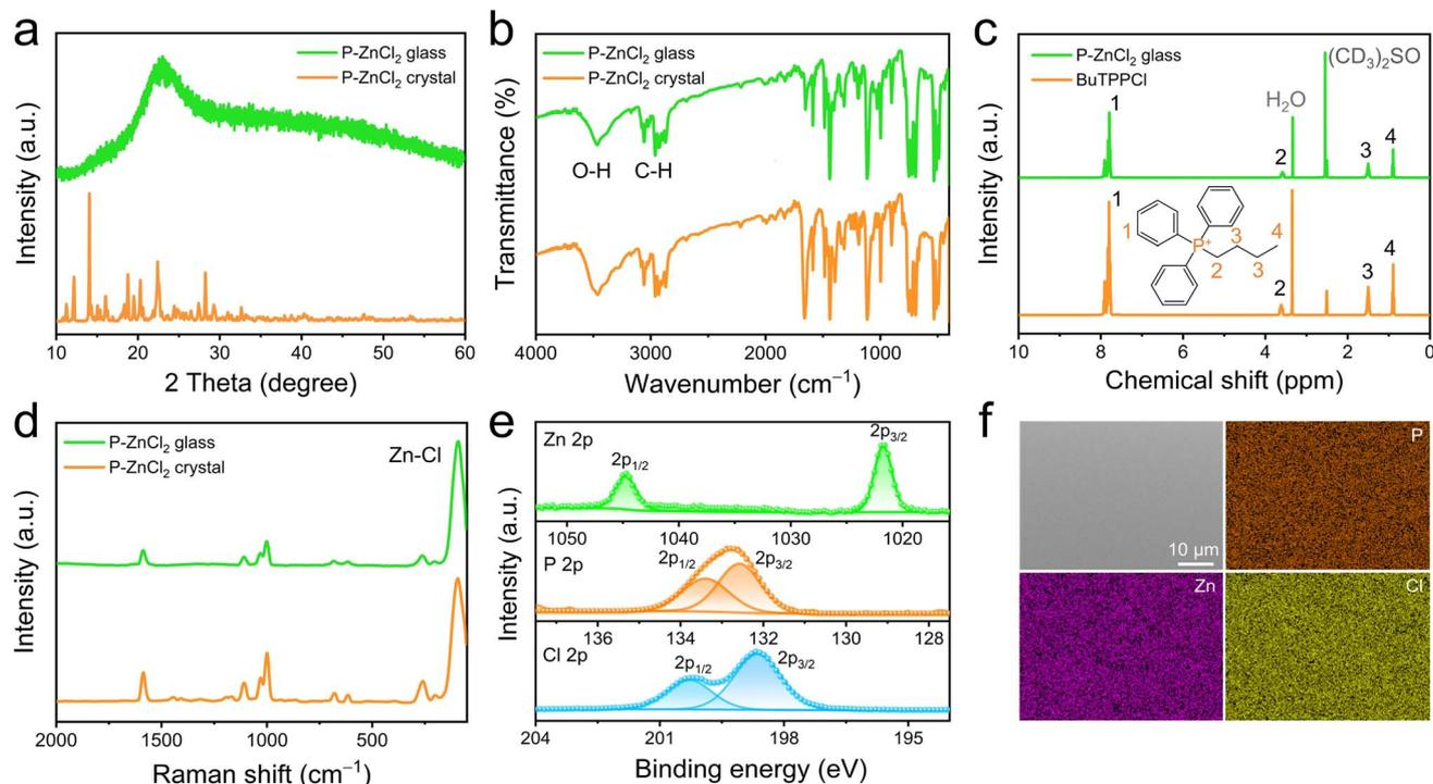
Fig. 2 (a) PXRD patterns of P-ZnCl<sub>2</sub> glass and crystal. (b) FTIR spectra of P-ZnCl<sub>2</sub> glass and crystal. (c) <sup>1</sup>H NMR spectra of P-ZnCl<sub>2</sub> glass and BuTPP<sup>+</sup> molecule. (d) Raman spectra of P-ZnCl<sub>2</sub> glass and crystal. (e) High-resolution XPS spectra of Zn 2p, P 2p, and Cl 2p in P-ZnCl<sub>2</sub> glass. (f) SEM image and EDS elemental mapping of P, Zn, and Cl in P-ZnCl<sub>2</sub> glass.
