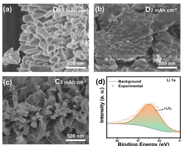
Fig. 6 (a and b) SEM images of Zn-HHTP electrodes at different discharge depths ( $0.8 \text{ mA h cm}^{-2}$  and  $2 \text{ mA h cm}^{-2}$ ). (c) SEM image of Zn-HHTP electrodes after charging to a depth of  $2 \text{ mA h cm}^{-2}$ . (d) Li 1s spectrum of the Zn-HHTP positive electrode discharged to  $2 \text{ mA h cm}^{-2}$ .
