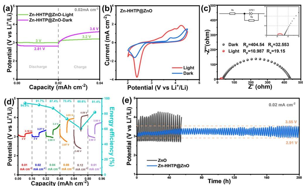
Fig. 5 Electrochemical performance test of Zn-HHTP@ZnO cathode in light/dark condition. (a) First discharge-charge curves of the battery at a current density of 0.02 mA cm<sup>-2</sup>, with a capacity limit of 0.02 mA h cm<sup>-2</sup>. (b) Cyclic voltammograms with a scan rate of 0.5 mV s<sup>-1</sup>. (c) EIS graph. (d) Charge-discharge curves of Zn-HHTP@ZnO cathode at different current densities. (e) Comparison of cycling performance of Zn-HHTP@ZnO cathode under light/dark conditions.
