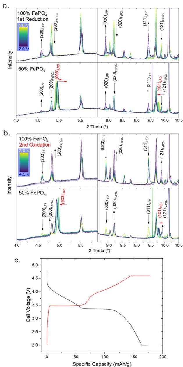
Fig. 7 (a) Evolution of the diffraction patterns for pure FePO<sub>4</sub> and 50% FePO<sub>4</sub>:LRO throughout the first reduction, from yellow line (4.8 V) to blue line (2.0 V), (b) same plot for the 2nd oxidation from yellow (2.0 V) to blue line (4.5 V). (c) Specific capacity vs. potential curves of the depicted *operando* experiments.
