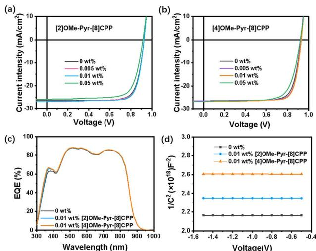
Fig. 4  $J-V$  plots of (a) [2]OMe-Pyr-[8]CPP and (b) [4]OMe-Pyr-[8]CPP, (c) EQE curves and (d) Mott-Schottky plot ( $1/C^2 - V$ ) of 0.01 wt% [2]OMe-Pyr-[8]CPP and [4]OMe-Pyr-[8]CPP, respectively.
