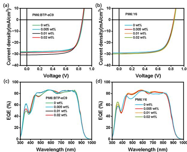
Fig. 6 (a)  $J$ - $V$  plots and (c) EQE curves of the PM6:BTP-eC9-based OSCs containing different concentrations of the [4]OMe-Pyr-[8]CPP dopant. (b)  $J$ - $V$  plots and (d) EQE curves of the PM6:Y6-based OSCs containing different concentrations of the [4]OMe-Pyr-[8]CPP dopant.
