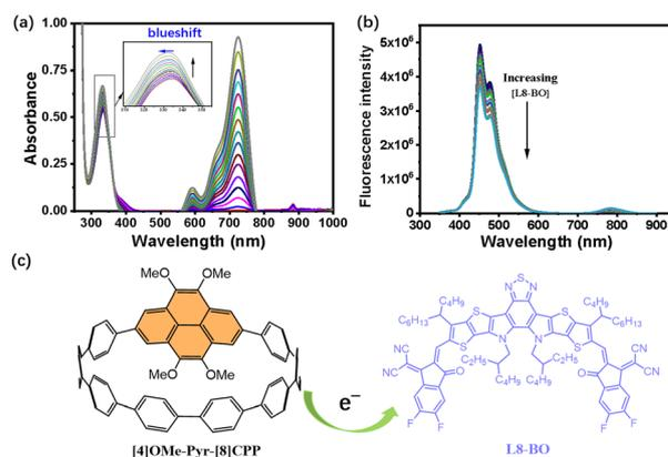
**Fig. 5** (a) Absorption spectral change upon titration of [4]OMe-Pyr-[8]CPP (conc.  $2.5 \times 10^{-6}$  M) with L8-BO (0–1.5 eq.) in CH<sub>2</sub>Cl<sub>2</sub> at 298 K. (b) Fluorescence emission spectral change upon titration of [4]OMe-Pyr-[8]CPP (conc.  $5.0 \times 10^{-7}$  M) with L8-BO (0–2.0 eq.) in CH<sub>2</sub>Cl<sub>2</sub> at 298 K ( $\lambda_{ex}$  = 330 nm). (c) Schematic illustration of electron transfer from [4]OMe-Pyr-[8]CPP to L8-BO.
