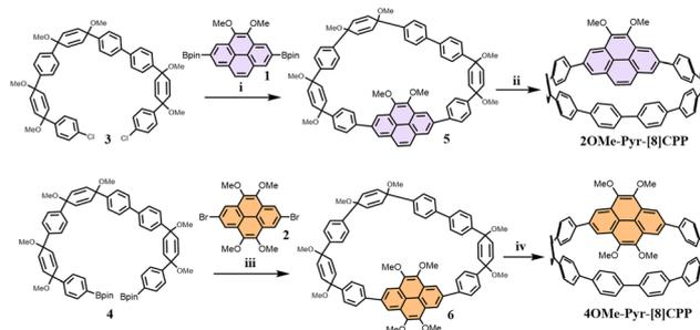
Scheme 1 Synthesis of nano hoops [2]OMe-Pyr-[8]CPP and [4]OMe-Pyr-[8]CPP. (i). SPhos Pd G2, K<sub>3</sub>PO<sub>4</sub>, dioxane/H<sub>2</sub>O, 80 °C, 2d, (ii). SnCl<sub>2</sub>, HCl, THF, 30% yield over two steps. (iii). SPhos Pd G3, K<sub>3</sub>PO<sub>4</sub>, dioxane/H<sub>2</sub>O, 80 °C, 2d, (iv). SnCl<sub>2</sub>, HCl, THF, 27% yield over two steps.
