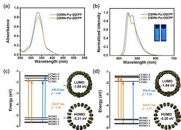
Fig. 3 (a) UV-vis and (b) fluorescence spectra of [2]OMe-Pyr-[8]CPP and [4]OMe-Pyr-[8]CPP in dichloromethane ( $c = 1.0 \times 10^{-5} \text{ M}$ ). Photograph of their fluorescence under 365 nm using a UV lamp (inset). Energy diagrams and pictorial representations of the frontier molecular orbitals for (c) [2]OMe-Pyr-[8]CPP and (d) [4]OMe-Pyr-[8]CPP calculated using TD-DFT.
