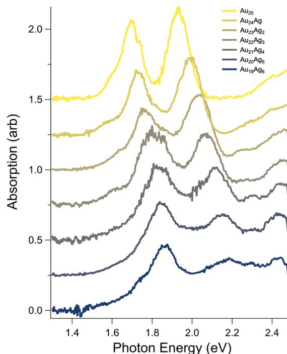
Fig. 3 Evolution of the spectra of  $\text{Au}_{25-n}\text{Ag}_n(\text{SC}_6\text{H}_{13})_{18}^-$  ( $n = 0-6$ ) atomically-precisely separated by mass spectrometry. Most spectral features blue shift with increasing Ag content, but the apparent HOMO–LUMO transition shows more complex behavior.
