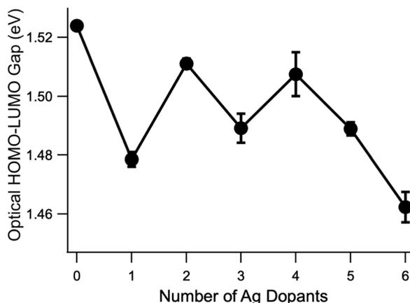
Fig. 4 Evolution of the extrapolated optical HOMO–LUMO gap as a function of the number of dopant Ag atoms. Error bars as shown represent the uncertainty of the fit performed to determine the  $x$ -intercept of the linear extrapolation. Details of the procedure to extract these values are given in the SI. An odd-even red/blueshifting pattern is observed for the first five doped clusters.
