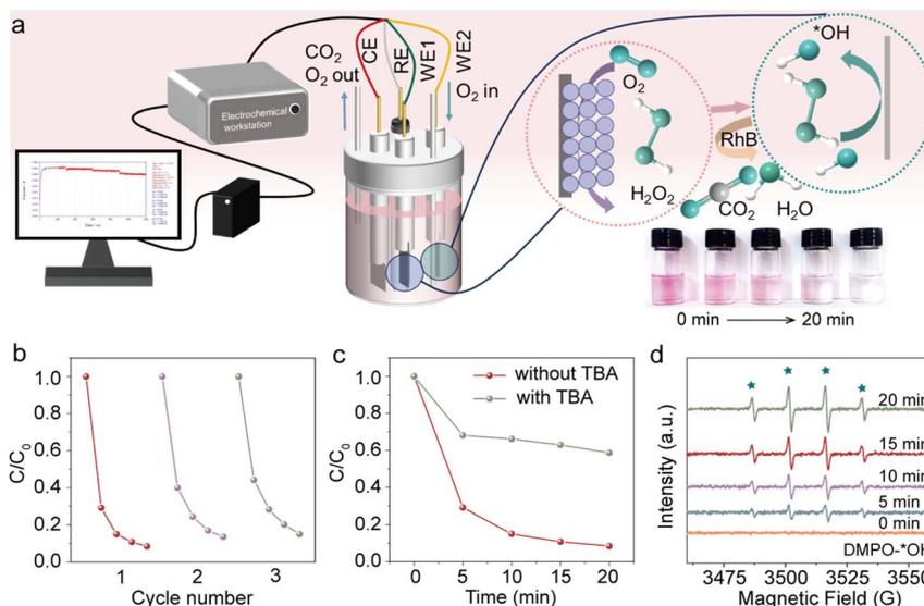
Fig. 5 (a) Schematic illustration of a dual cathode configuration for the degradation of RhB. (b) RhB degradation comparison rate *versus* cycle number using Co-CuS<sub>ED</sub> as the catalyst. (c) RhB degradation efficiency with/without *tert*-butanol (TBA). (d) EPR spin trapping with dimethyl pyridine *N*-oxide (DMPO) at 0, 5, 10, 15, and 20th minute operation using Co-CuS<sub>ED</sub> as the catalyst.
