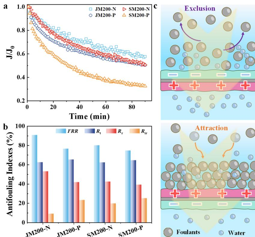
Fig. 7 Anti-fouling performance of the membranes. Normalized flux (a) and fouling resistance (b) of the Janus and single-sided membranes after fouling by BSA ( $100 \text{ mg L}^{-1}$ ). Anti-fouling mechanism of the Janus membrane from different feed directions (c).
