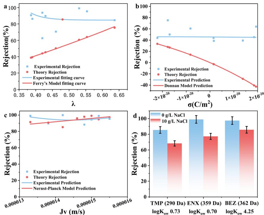
Fig. 5 Experimental and theoretical data for TC rejection by membrane fitting with Ferry's model (a), the Donnan model (b) and the Donnan-Steric pore model (c).  $\lambda$  is the relative size parameter defined as the ratio of the solute size to the membrane pore size,  $\sigma$  is the charge density (C m<sup>-2</sup>), and  $J_v$  is the volumetric flux (m s<sup>-1</sup>). Rejection of typical EOCs by JM200 at high salinity (10 g per L NaCl) (d).
