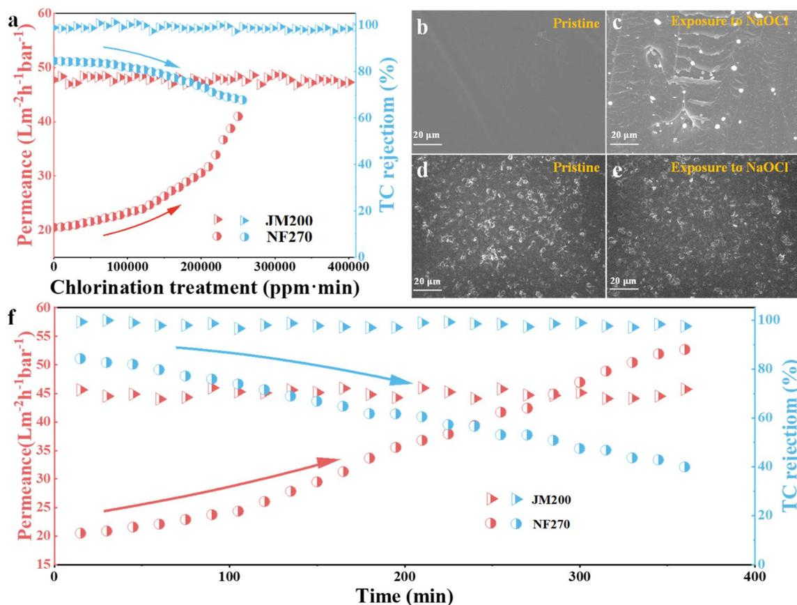
Fig. 8 Chlorine resistance of the membranes. Separation performance of JM200 and NF270 after exposure to NaOCl solution at neutral pH for filtration of TC (a), SEM images of the NF270 (b and c) and JM200 (d and e) surfaces before and after exposure to NaOCl, and dynamic cross-flow chlorine resistance tests of JM200 and NF270 for filtration of TC solution containing NaClO ( $50 \text{ mg L}^{-1}$ ) under a pressure of 0.2 MPa (f).
