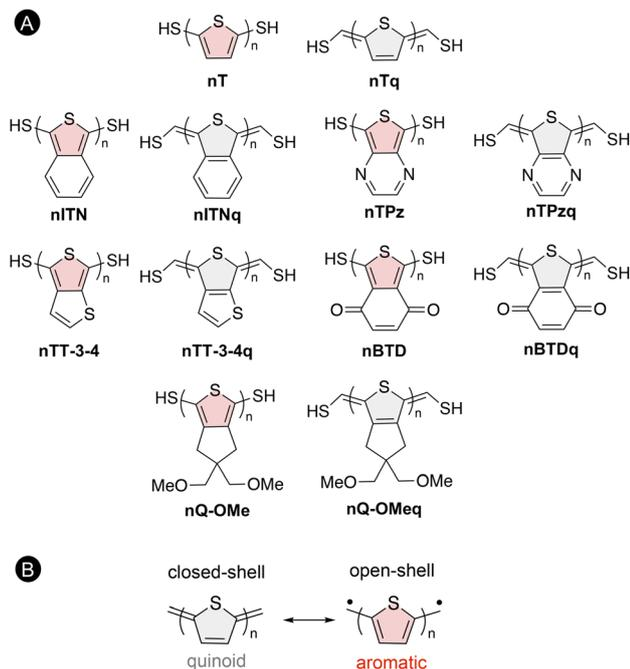
**Scheme 1** (A) Oligothiophenes selected to assess the interplay between diradical character, aromaticity, and conductance. The quinoidal oligothiophenes are indicated by the suffix “q”. The oligomer chain  $n$  varies from one to six monomer units. (B) Quinoidal and aromatic resonance structures proposed for the singlet ground state of quinoidal oligothiophenes.
