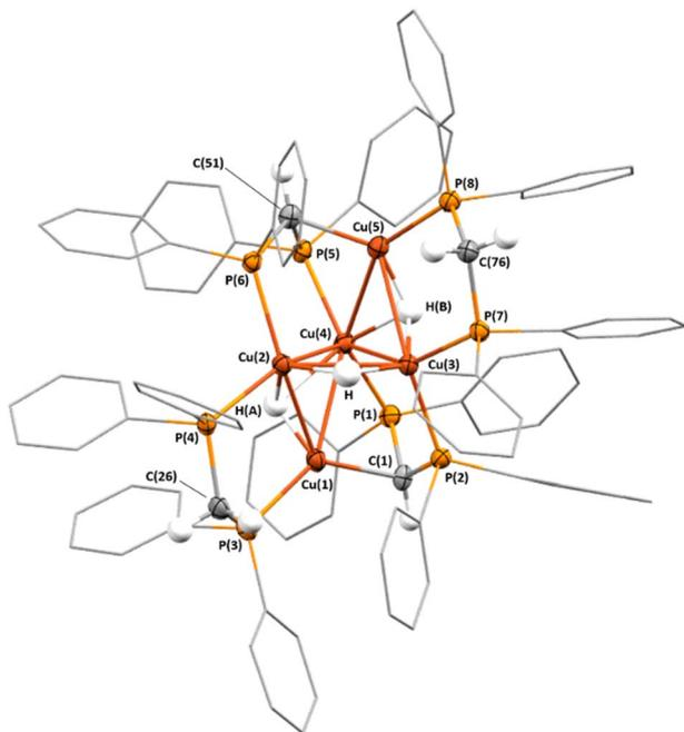
Fig. 2 Illustration of the solid-state structure of **2·4benzene** obtained from single crystal X-ray diffraction experiments. Displacement ellipsoids are drawn with 50% probability, and carbon atoms of the *P*-phenyl groups are drawn wireframe. For clarity, only one of two molecules in the asymmetric unit are depicted, and hydrogen atoms, aside for the bridging hydride ligands and methylene/methine protons, and lattice solvent are omitted.
