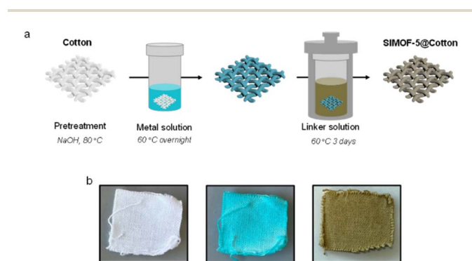
Fig. 6 (a) Schematic preparation of SIMOF-5@cotton composite. (b) Photographs of pristine cotton fabric, copper acetate coated cotton fabric and SIMOF-5@cotton composite.
