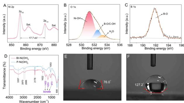
Fig. 2 (A) Ni 2p spectra, (B) O 1s spectra, and (C) B 1s spectra of BI-Ni(OH)<sub>2</sub> nanosheets. (D) FT-IR spectra of BI-Ni(OH)<sub>2</sub> and P-Ni(OH)<sub>2</sub> nanosheets. Water contact angle tests of (E) BI-Ni(OH)<sub>2</sub> and (F) P-Ni(OH)<sub>2</sub> nanosheets.
