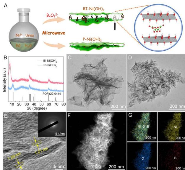
Fig. 1 (A) Schematic illustration of the synthesis of BI-Ni(OH)<sub>2</sub> and P-Ni(OH)<sub>2</sub> nanosheets. (B) XRD patterns of BI-Ni(OH)<sub>2</sub> and P-Ni(OH)<sub>2</sub> nanosheets. (C) TEM image of P-Ni(OH)<sub>2</sub> nanosheets. (D) TEM, (E) HRTEM (inset: the SAED pattern), (F) HAADF-STEM, and (G) EDX elemental mapping images of BI-Ni(OH)<sub>2</sub> nanosheets.
