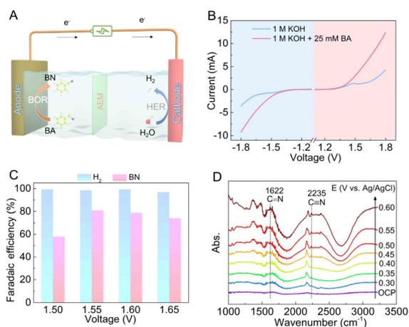
Fig. 4 (A) Schematic illustration of the BOR paired with the HER over a two-electrode electrolyzer. (B) LSV curves recorded at a scan rate of 5 mV s<sup>-1</sup> in 1.0 M KOH with and without 25 mM BA. (C) The calculated FEs for H<sub>2</sub> and BN production at different voltages in the two-electrode electrolyzer. (D) Potential-dependent *in situ* FT-IR spectra of the BI-Ni(OH)<sub>2</sub> catalyst in 1.0 M KOH with 25 mM BA.
