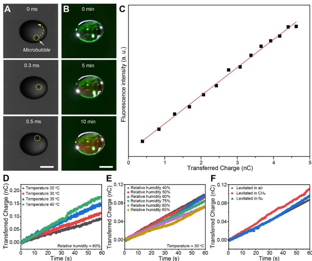
Fig. 2 (A) A microbubble rotating at high speed in the droplet. (B) Increase of fluorescence emission of the droplet depended on levitated time. (C) Lineal relationship between fluorescence intensity and transferred charge of the droplet. (D) Transferred charge increase at different environmental temperatures. (E) Transferred charge increase at different relative humidity. (F) Transferred charge increase in different atmosphere. The scale bars are 1 mm for both panel A and B.
