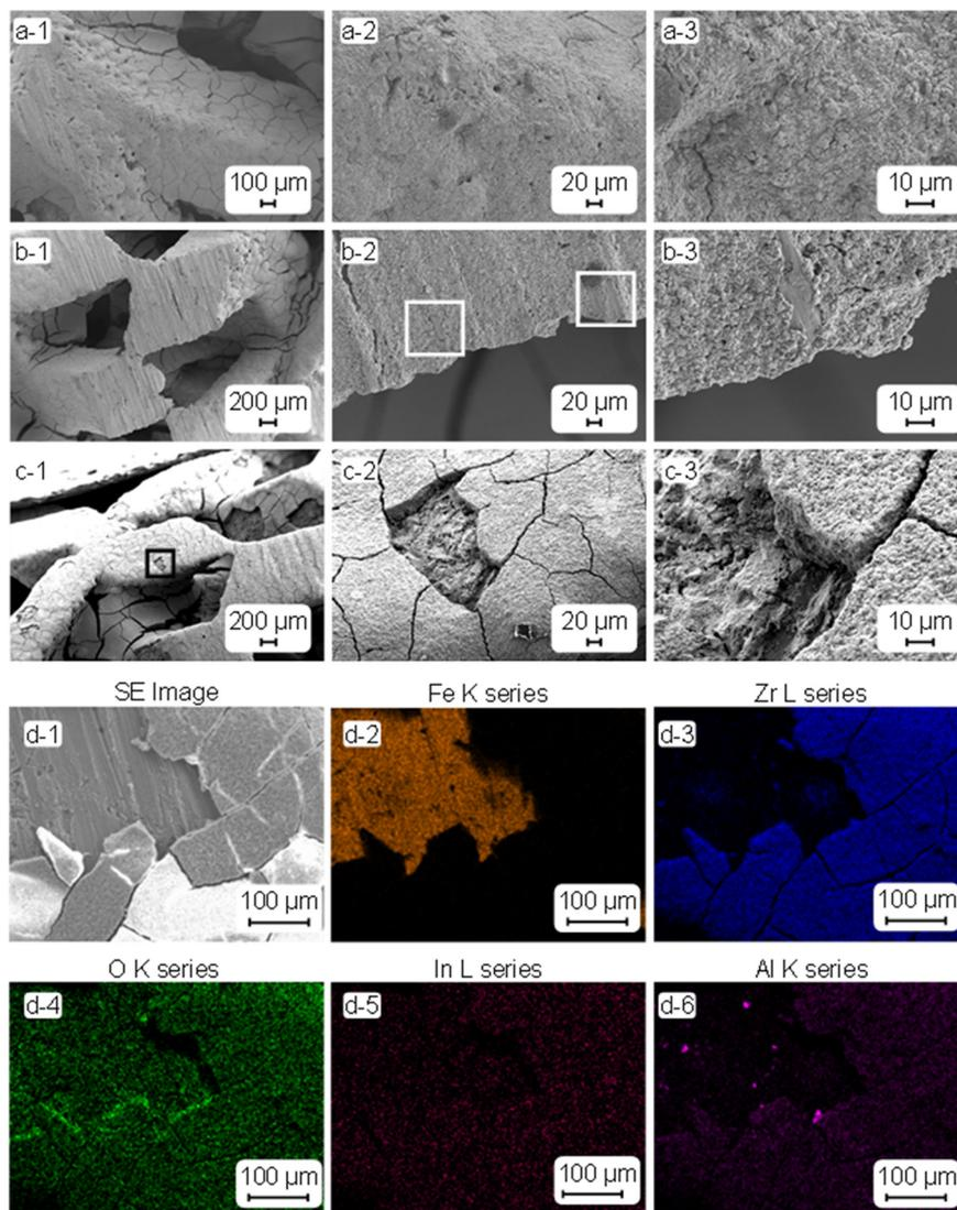
**Fig. 2** SEM images showing an evenly coated surface (a), uncoated spots on the outer region of the CSM (b), and cracks and small defects of the coating (c) and SEM-EDXS images (d2–d6 show different elements) of a spot showing the CSM scaffold and the In<sub>2</sub>O<sub>3</sub>/ZrO<sub>2</sub> coating (d). Images 1–3 in the rows a–c show the microscopic images at different scales.
