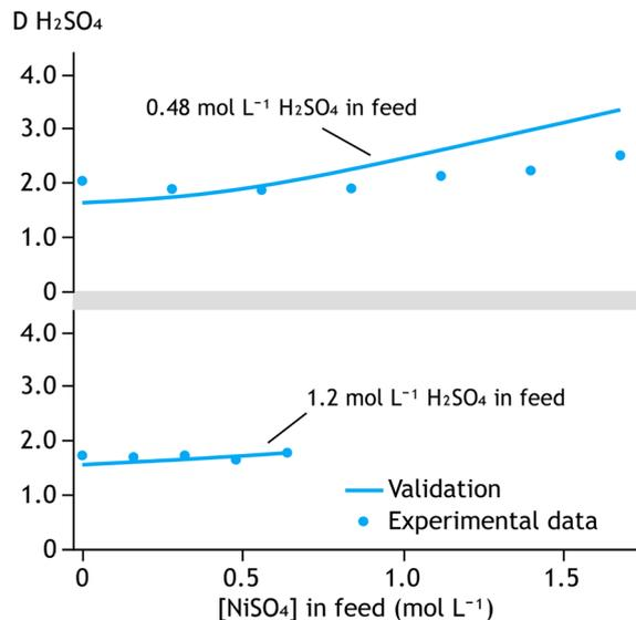
Fig. 16 Validation calculation (line) of experimental data (markers) on H<sub>2</sub>SO<sub>4</sub> recovery from NiSO<sub>4</sub> solutions by 40 vol% TEHA in 1-octanol at 25 °C.
