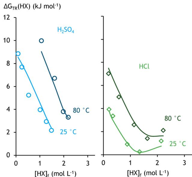
Fig. 11 Model fit of  $\text{H}_2\text{SO}_4$  and HCl extraction by 43 vol% TEHA diluted in *n*-dodecane.<sup>47</sup>
