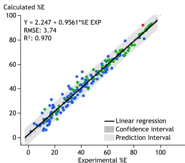
Fig. 13 Quality of fit graph for %  $E$  data of the synergistic system before (top) and after (bottom) optimisation. Statistical intervals are given with 95% confidence. The dashed grey line represents the ideal fit.
