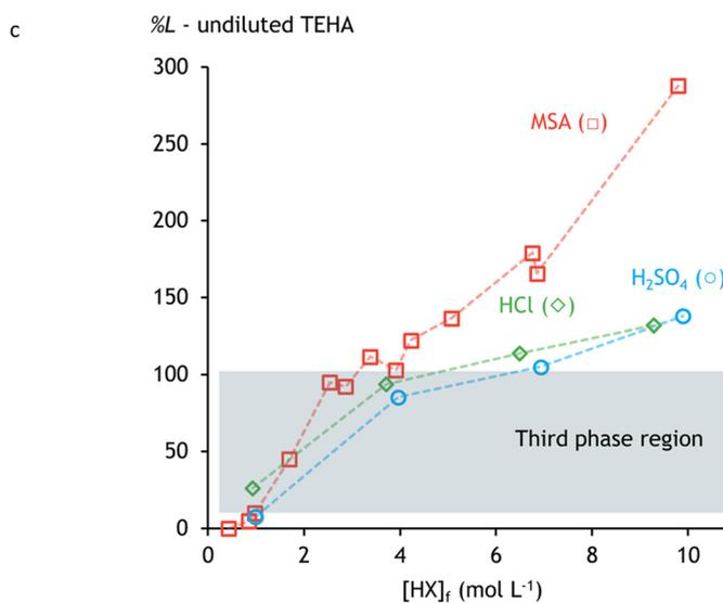
Fig. 1 Solvent extraction data of H<sub>2</sub>SO<sub>4</sub>, HCl, and MSA – undiluted 1-octanol systems at 25 °C. Distribution ratios (a), volume changes (b), and organic phase densities (c) are shown.
