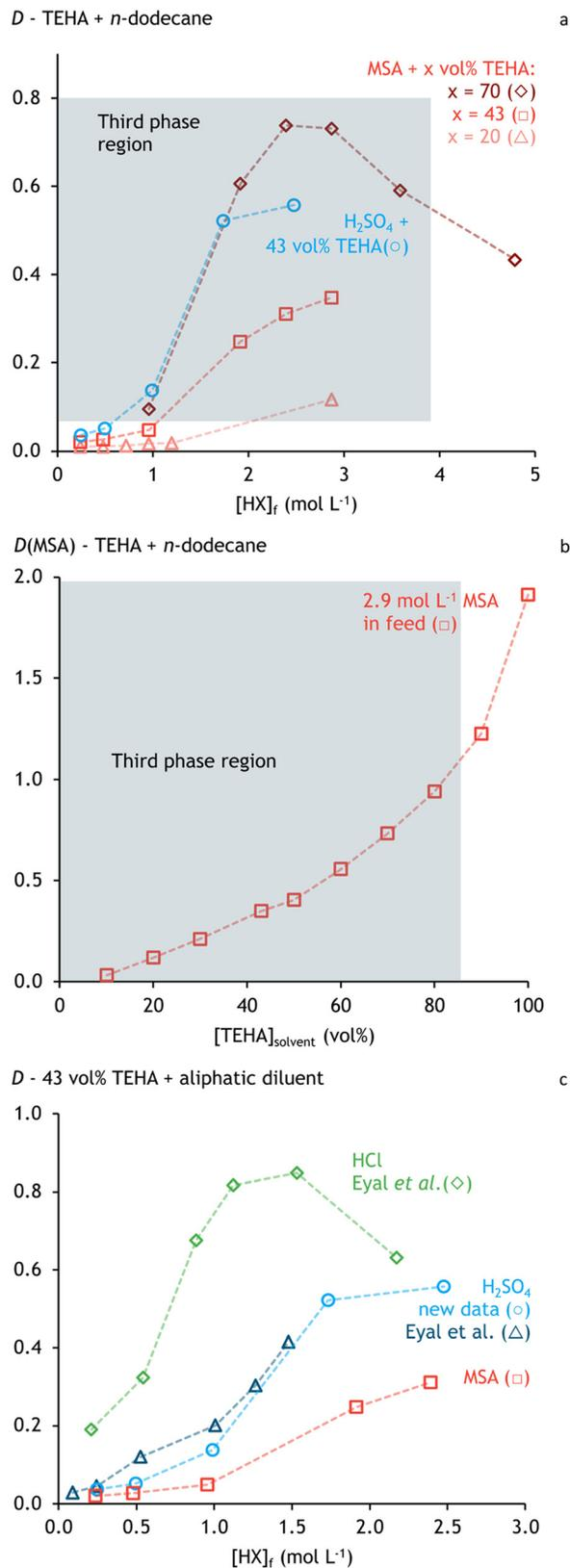
Fig. 3 Solvent extraction data of  $H_2SO_4$ , HCl, and MSA – TEHA + dodecane systems at 25 °C. Graph c compares this to literature data from Eyal et al.<sup>46</sup> Distribution ratios are shown for three TEHA concentrations with varying  $H_2SO_4$  concentrations in the feed (a), and with varying initial TEHA concentrations in the solvent (b). (c) Compares the extraction of HCl,  $H_2SO_4$ , MSA by 43 vol% TEHA.
