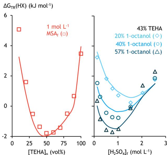
Fig. 14 Model fit (lines) of MSA and  $\text{H}_2\text{SO}_4$  extraction mixtures of TEHA and 1-octanol (left) and 43 vol% TEHA in mixtures of 1-octanol and *n*-dodecane (right).<sup>14,42</sup>
