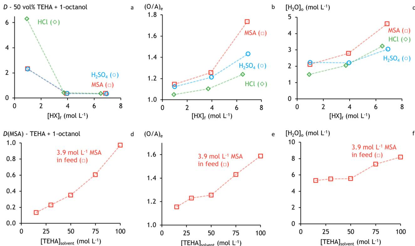
Fig. 4 Solvent extraction data of H<sub>2</sub>SO<sub>4</sub>, HCl, and MSA – TEHA + 1-octanol systems at 25 °C. Systems depicted in a to c contain 50 vol% TEHA in 1-octanol, and in d to f contain a variable amount of TEHA in 1-octanol. Distribution ratios (a and d), volume changes (b and e), and water uptake by the solvent (c and f) are shown.
