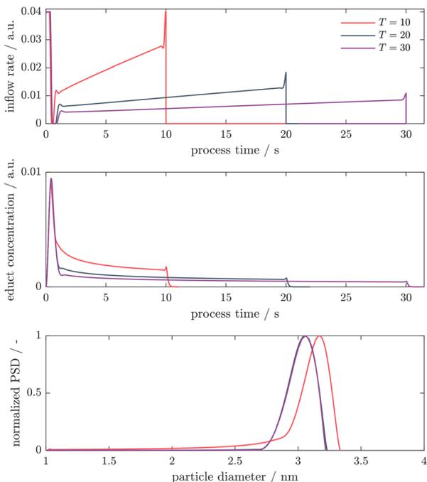
**Fig. 3** Variation of final inflow time  $T_c$  from 10 to 30 while the upper bound  $u_{\max} = 0.04$  and regularization parameter  $\kappa = 10^{-1}$  is chosen constant. There is a clear influence of shorter times, i.e.  $T_c = 10$  on the width of the final PSD (red, lower figure) as the nucleation phase and growth phase cannot be “separated” as needed, whereas there is only a minor gain when increasing  $T_c$  from 20 to 30.
