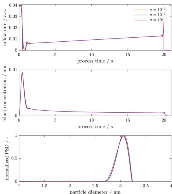
**Fig. 6** Increasing the  $H^1$ -regularization from  $\kappa = 10^{-2}$  to  $10^0$  results in a control with increasing regularity (left plot) and causes an increase in the standard deviation of the resulting PSD (lower figure). The final inflow time  $T_c = 20$  and upper bound  $u_{\max} = 0.04$  are chosen to be constant.
