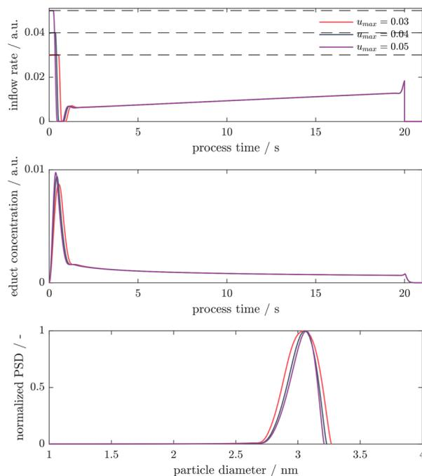
**Fig. 4** Limiting the maximal inflow rate  $u(t) \leq u_{\max} \forall t \in [0, T]$ . The effect on the final PSD (lower figure) is only minor and there is for decreasing  $u_{\max}$  only a slight widening of the PSD visible. The final inflow time  $T_c = 20$  and regularization parameter  $\kappa = 10^{-1}$  are chosen to be constant.
