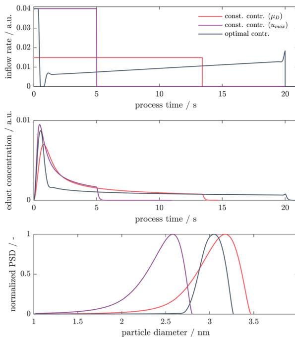
**Fig. 1** Comparison of two constant controls (red and purple) with the optimized control (black). The constant controls are chosen in red: such that the final PSD possesses the desired mean size  $\mu_D = 3$  and in purple: to showcase a shorter injection time, showing that reducing the injection time reduces the mean size. This highlights the benefit of the time-dependent control, which clearly shows a smaller standard deviation of the final PSD.
