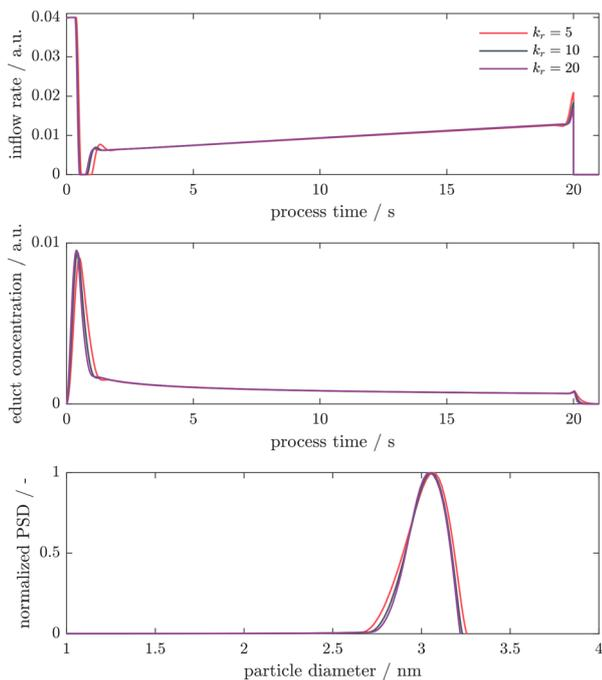
**Fig. 5** The reduction rate was varied as  $k_r \in \{5, 10, 20\}$ . At lower reduction rates, the inflow rate is controlled more indirectly, leading to a sub-optimal reactant concentration profile and, as a result, a broader PSD.
