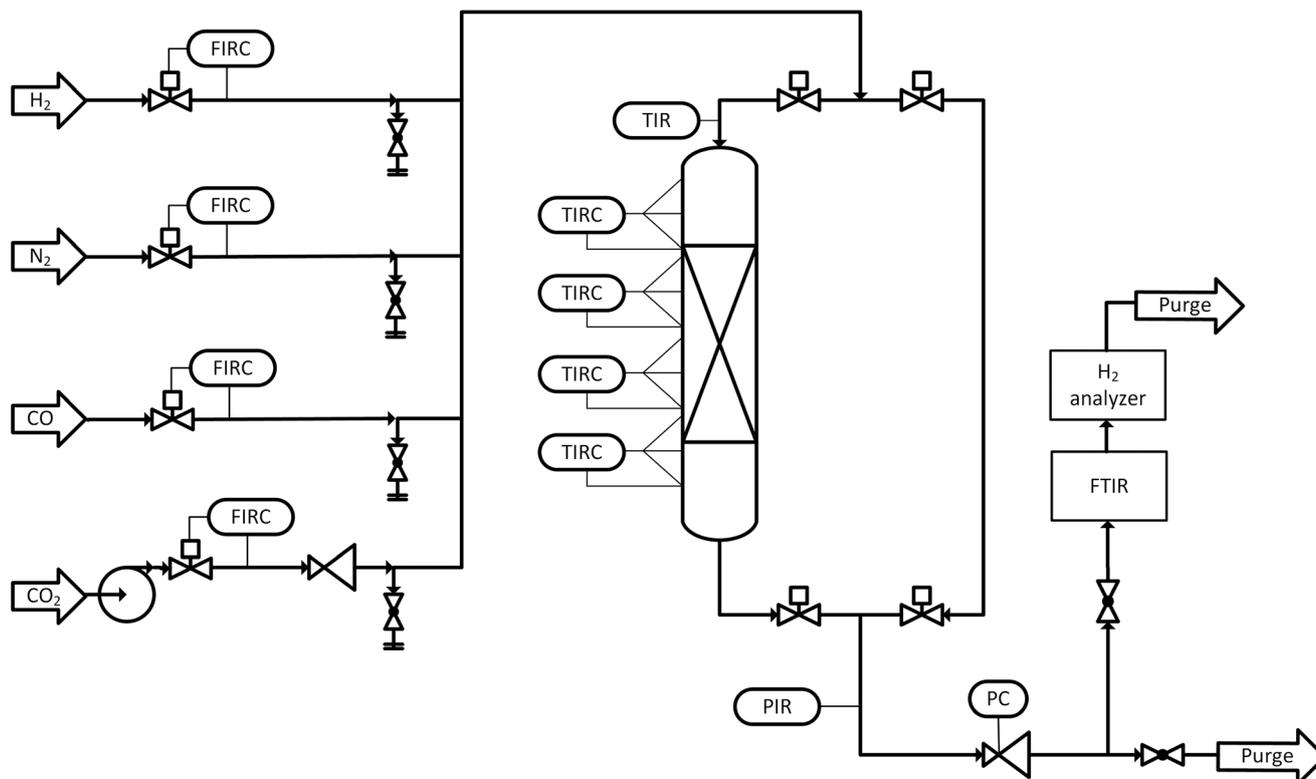
Fig. 2 Schematic flowchart of the reactor setup.
