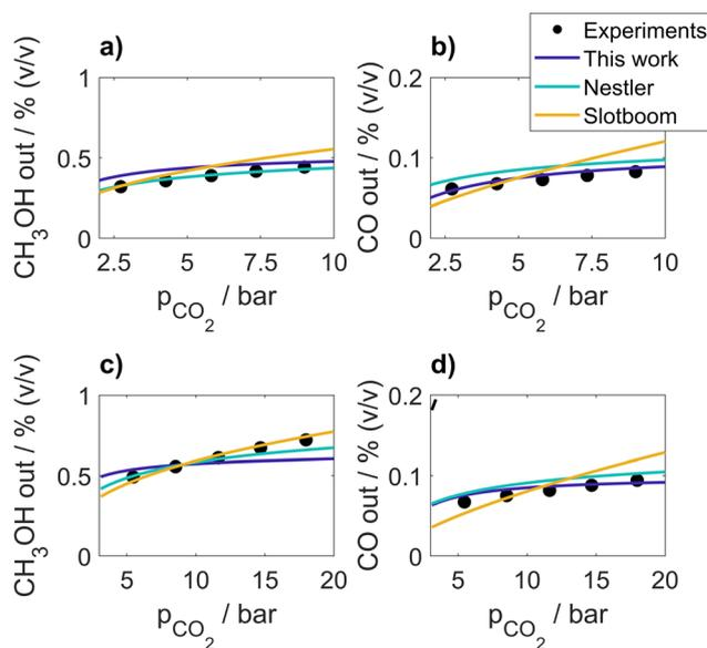
Fig. 7 Variations in  $\text{CO}_2$  partial pressure for the following conditions:  $y_{\text{H}_2,\text{in}} = 0.59$ ,  $T = 210 \text{ °C}$ ,  $\text{SV} = 72 \text{ Nm}^3 \text{ kg}_{\text{cat}}^{-1} \text{ h}^{-1}$ , (a and b)  $p = 31 \text{ bar}$ , (c and d)  $p = 62 \text{ bar}$ .
