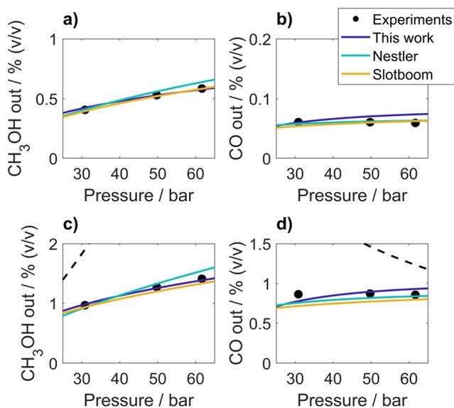
Fig. 5 Variations in pressure for the following conditions:  $y_{\text{CO}_2,\text{in}} = 0.18$ ,  $y_{\text{H}_2,\text{in}} = 0.59$ ,  $\text{SV} = 48 \text{ Nm}^3 \text{ kg}_{\text{cat}}^{-1} \text{ h}^{-1}$ , (a and b)  $T = 200 \text{ °C}$ ; (c and d)  $T = 240 \text{ °C}$ . Dashed line represents thermodynamic equilibrium.
