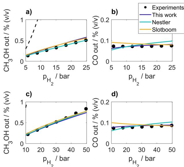
Fig. 6 Variations in  $\text{H}_2$  partial pressure for the following conditions:  $y_{\text{CO}_2,\text{in}} = 0.18$ ,  $T = 210 \text{ °C}$ ,  $\text{SV} = 72 \text{ Nm}^3 \text{ kg}_{\text{cat}}^{-1} \text{ h}^{-1}$ , (a and b)  $p = 31 \text{ bar}$ , (c and d)  $p = 62 \text{ bar}$ . Dashed line represents thermodynamic equilibrium.
