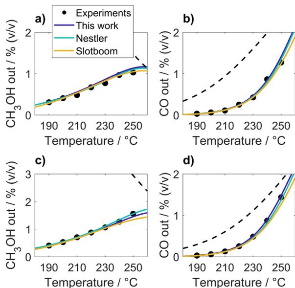
Fig. 4 Variations in temperature for the following conditions:  $y_{\text{CO}_2,\text{in}} = 0.18$ ,  $y_{\text{H}_2,\text{in}} = 0.59$ ,  $\text{SV} = 48 \text{ Nm}^3 \text{ kg}_{\text{cat}}^{-1} \text{ h}^{-1}$ , (a and b)  $p = 31 \text{ bar}$ ; (c and d)  $p = 50 \text{ bar}$ . Dashed line represents thermodynamic equilibrium.
