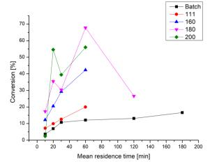
Fig. 7 Diels-Alder reaction for conversion to 3 at different temperatures and reaction times.
