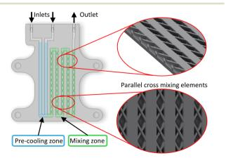
Fig. 3 Microreactor with a pre-cool zone and mixing zone with parallel cross mixing channels.
