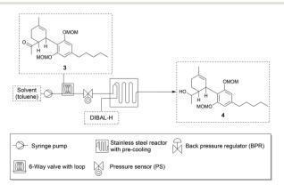
Scheme 2 Reduction to alcohol 4 under continuous flow conditions.
