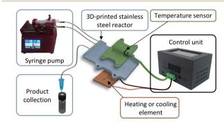
Fig. 1 Schematic of the microfluidic system.
