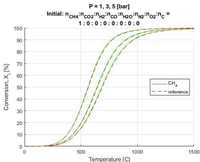
Fig. 1 Comparison of CH<sub>4</sub> conversion profiles calculated using the Gibbs minimization method and those calculated using eqn (32) taken from ref. 33 at pressures of 1, 2, and 5 bar.
