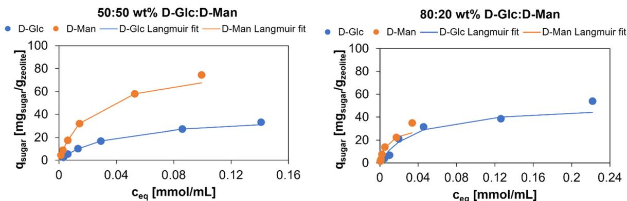
**Fig. 6** Competitive adsorption of D-Glc and D-Man by CaY zeolites. Adsorption conditions: 500 mg zeolite, 3 mL 70:30 wt% EtOH:H<sub>2</sub>O solution, 2 h, RT, 500 rpm.
