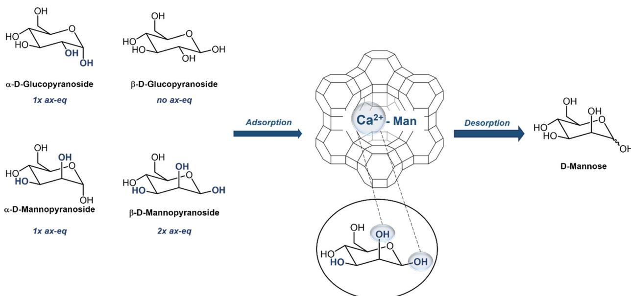
Fig. 2 Separation of D-Man *via* Ca<sup>2+</sup> complexation in CaY zeolite.
