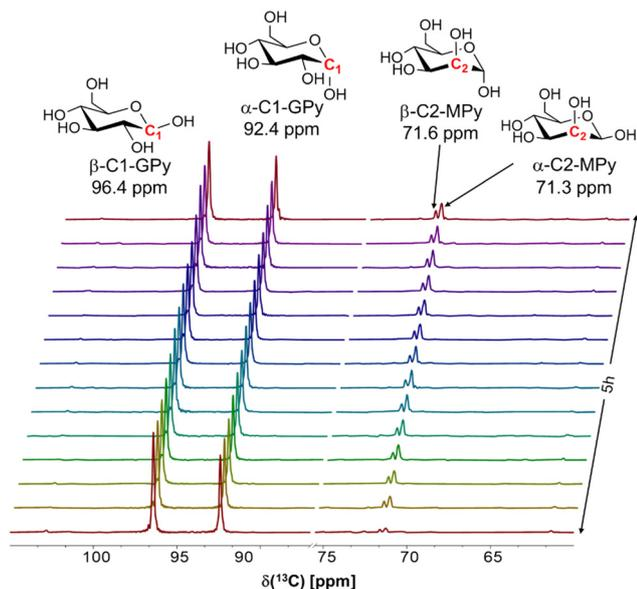
**Fig. 4** Direct polarization MAS solid-state  $^{13}\text{C}$  NMR (11.7 T, 3 kHz MAS) of Sn-OF-1 (9.4 mg) in the presence of a solution of 1- $^{13}\text{C}$ -D-Glc in 50:50 wt% EtOH:H<sub>2</sub>O (7.0 mol L<sup>-1</sup>, 0.195 mL) at 92 °C. The time-resolved *operando* spectra show conversion of D-Glc to D-Man.
