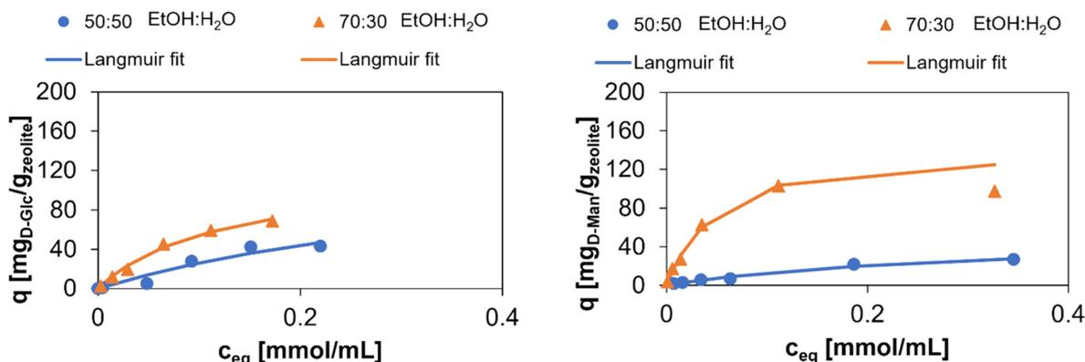
**Fig. 5** Adsorption isotherms for individually adsorbed D-Glc (left) and D-Man (right) on CaY zeolites at different EtOH:H<sub>2</sub>O ratios. Adsorption conditions: 500 mg zeolite, 3 mL EtOH:H<sub>2</sub>O solution, 2 h, RT, 500 rpm.
