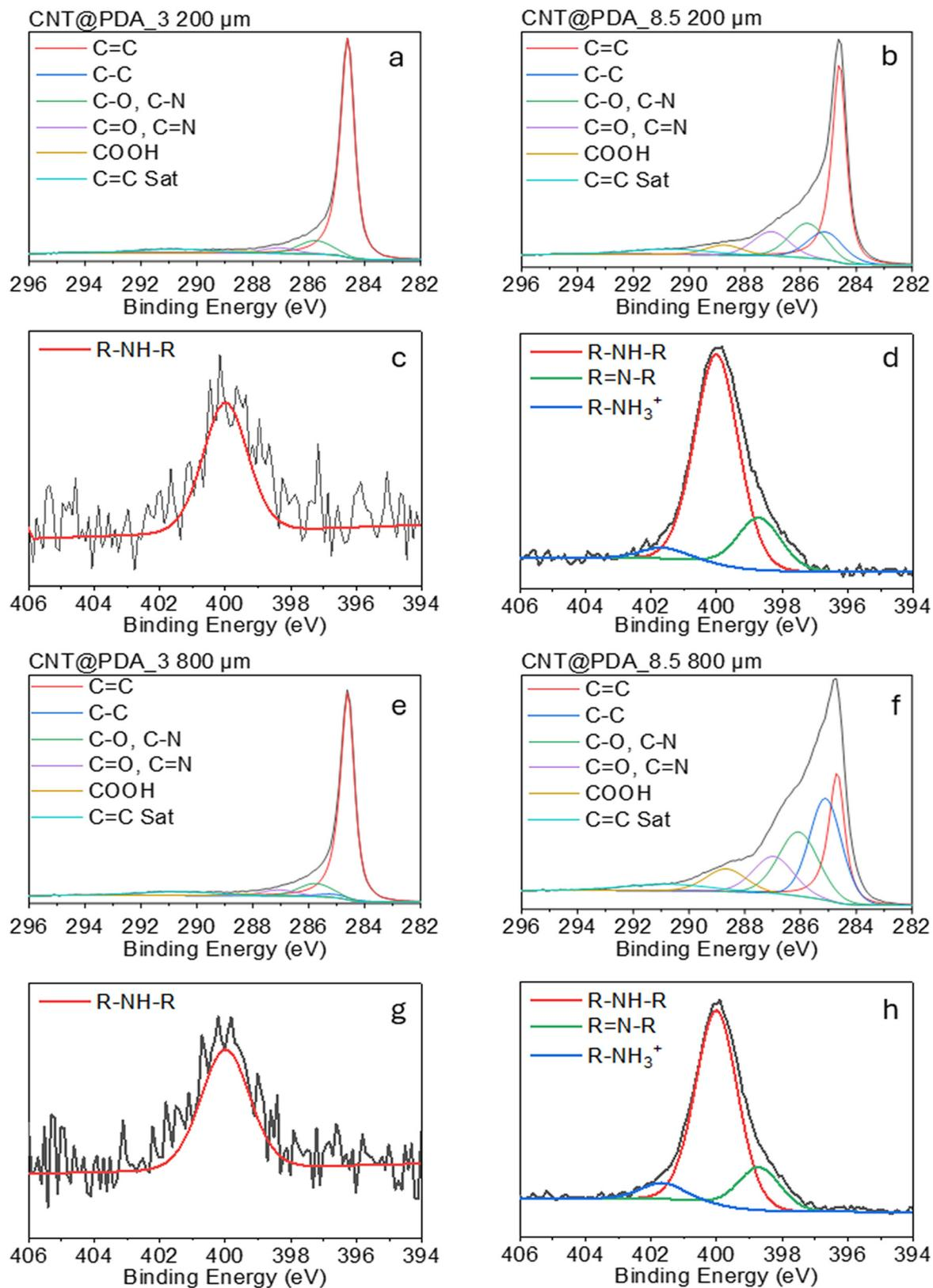
Fig. 2 High-resolution C 1s core level spectra of 200  $\mu\text{m}$  CNTs functionalized with (a) PDA at pH 3 and (b) PDA at pH 8.5, 800  $\mu\text{m}$  CNTs functionalized with (e) PDA at pH 3, (f) PDA at pH 8.5. High-resolution N 1s core level spectra of 200  $\mu\text{m}$  CNTs functionalized with (c) PDA at pH 3 and (d) PDA at pH 8.5, 800  $\mu\text{m}$  CNTs functionalized with (g) PDA at pH 3 and (h) PDA at pH 8.5.
