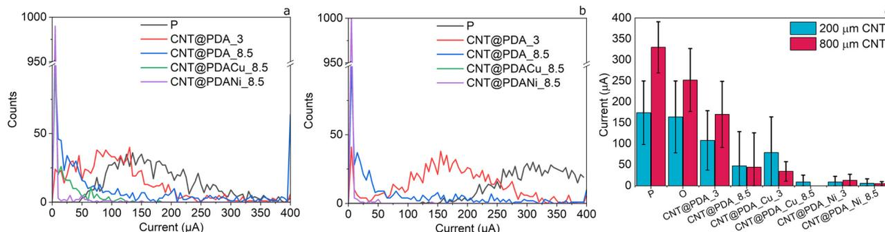
**Fig. 5** Distribution of current measured by C-AFM for 200 (a) and 800 (b) μm pristine CNTs, CNTs functionalized with PDA at pH 3 and 8.5, and in the presence of copper and nickel ions. Weighted average current values (c) of 200 and 800 μm pristine and oxidized CNTs, as well as CNTs functionalized with PDA at pH 3 and 8.5, and as well in the presence of copper and nickel ions. Error bars represent the standard deviation from six independent measurements per sample.
