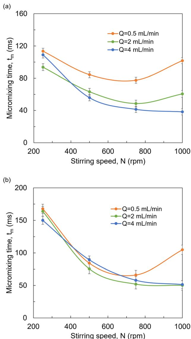
Fig. 7 Micromixing time,  $t_m$ , vs. stirring speed,  $N$ , for flowrates of  $Q = 0.5, 2$  and  $4$  mL min<sup>-1</sup> for (a) the slotted impeller and (b) the cross stir bar. Error bars are calculated based on the standard deviation of repeated experiments.
