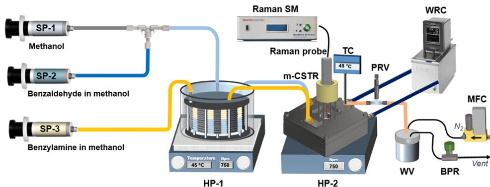
Fig. 4 Experimental set-up for the kinetic data acquisition of the *n*-benzylidenebenzylamine synthesis. SP: syringe pump SM: spectrometer, PRV: pressure relief valve, WRC: water circulator, HP: hotplate-stirrer, MFC: mass flow controller, TC: thermocouple, WV: waste vessel, BPR: back pressure regulator, m-CSTR: miniaturised CSTR. HP-2 was only used as a stirrer. All temperature, pressure and flow equipment were controlled by LabVIEW.
