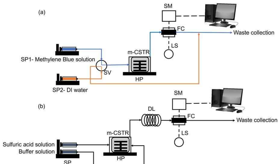
**Fig. 2** (a) Experimental set-up for the residence time distribution (RTD) studies (orange lines indicate the DI water flow and blue lines indicate the blue dye flow), (b) experimental set-up for the micromixing studies using the Villermaux–Dushman reaction. SP: syringe pump, SV: switch valve, SM: UV-vis spectrometer, FC: flow cell, LS: light source, DL: delay loop, HP: hotplate-stirrer, m-CSTR: miniaturised CSTR.
