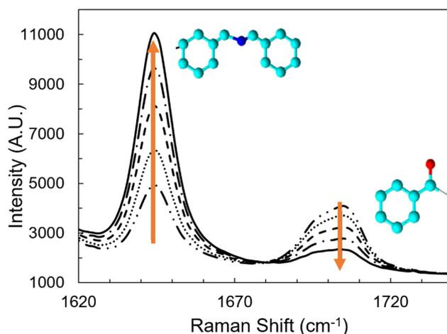
Fig. 5 Recorded Raman spectra of benzaldehyde (right peak) and *n*-benzylidenebenzylamine (left peak) as a function of residence time,  $\tau$ . Arrows indicate decreasing flowrates, i.e. increasing residence time.
