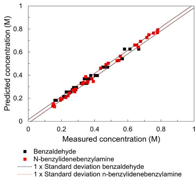
**Fig. 8** Parity plot for model predicted and experimentally measured reactor concentrations of benzaldehyde and *n*-benzylidenebenzylamine. The dashed lines represent the one-standard deviation limits.
