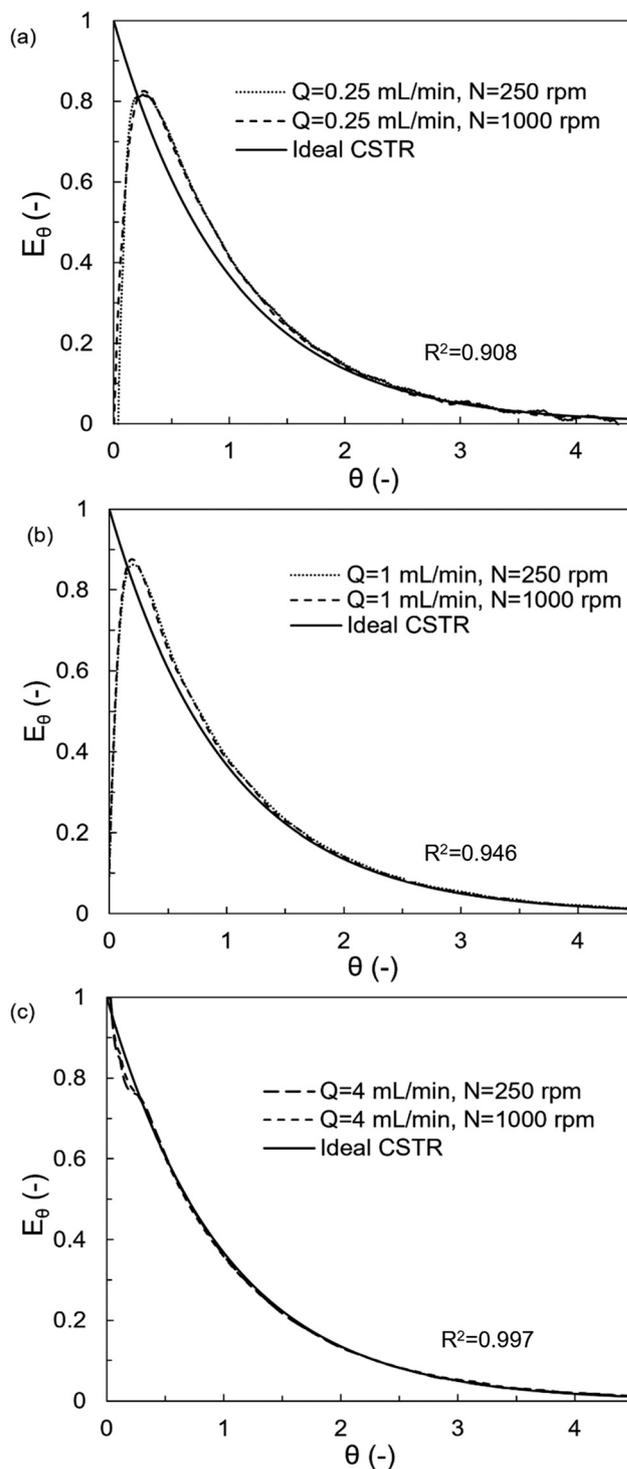
**Fig. 6**  $E_\theta$  curve of the m-CSTR (2.35 mL effective volume) for a total flowrate of (a) 0.25 mL min<sup>-1</sup> and (b) 1 mL min<sup>-1</sup> and (c) 4 mL min<sup>-1</sup> at 250 and 1000 rpm compared to the ideal CSTR model, using the slotted impeller.
