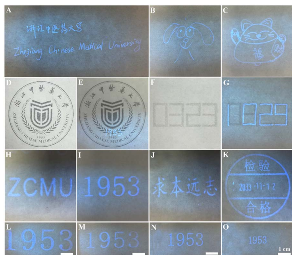
Fig. 6 (A–C) Depict samples handwritten on paper with a pen under UV light; (D–G) present a comparative display of numerals under natural light (left) and UV light (right); (H–K) exhibit photos of letters, numerals, Chinese characters, and intricate patterns made by stamps sequentially under UV light; (L–O) show images of the patterns fabricated using stamps of varying sizes, captured under UV light illumination.
