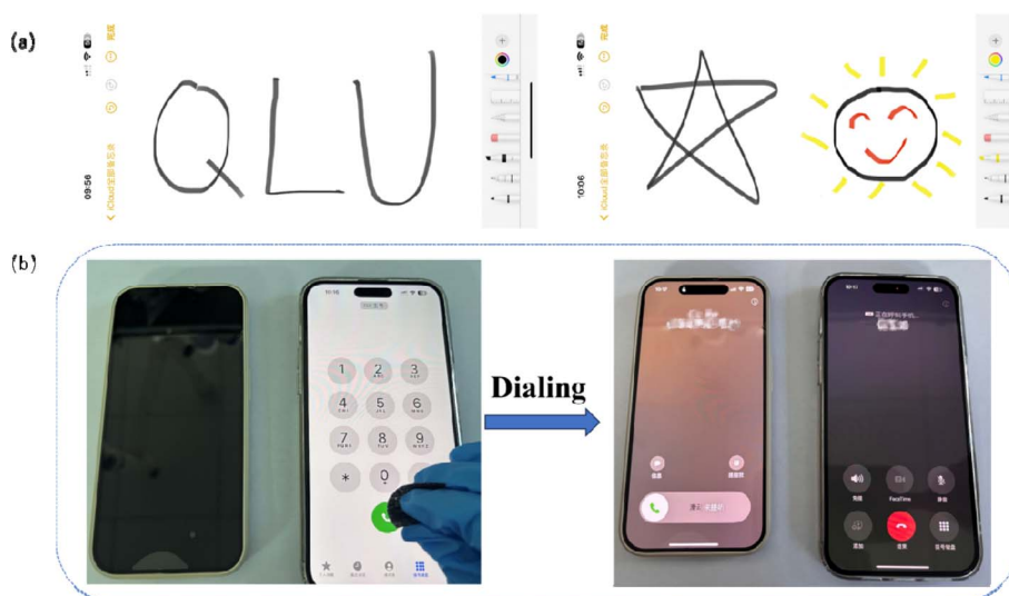
Fig. 12 (a) Handwriting “QLU” and drawing patterns such as a star and smiley sun; (b) dialing a phone number on a smartphone screen.
