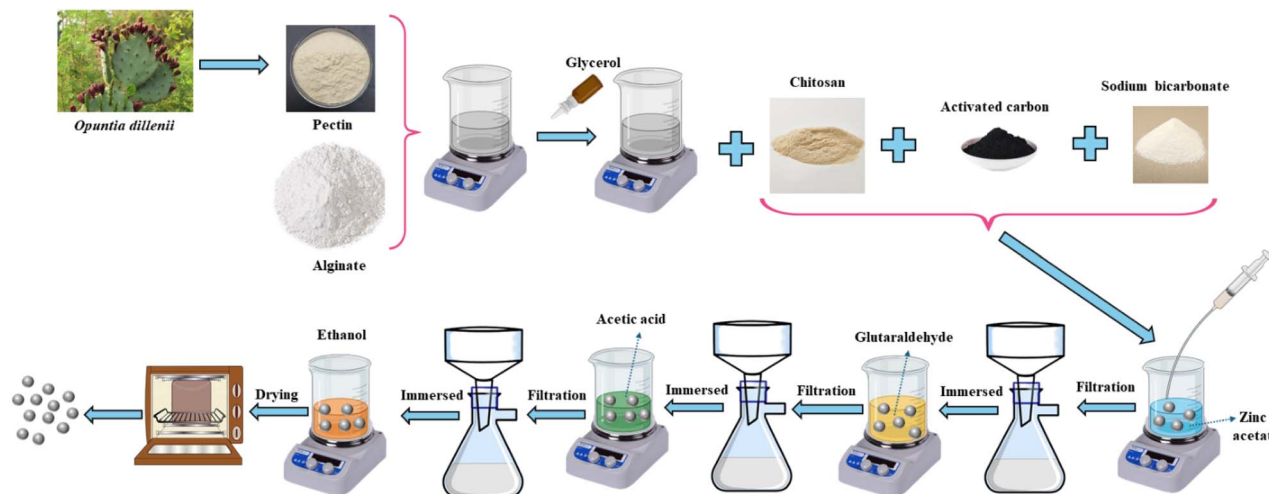
Fig. 1 Schematic representation of the stepwise fabrication process of SPCA composite beads derived from Opuntia dillenii biomass.
