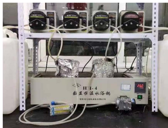
Fig. 1 Experimental setup: (a) Chlorella expansion, (b) bacteria–microalgae ratio, (c) aeration, and (d) light test.
