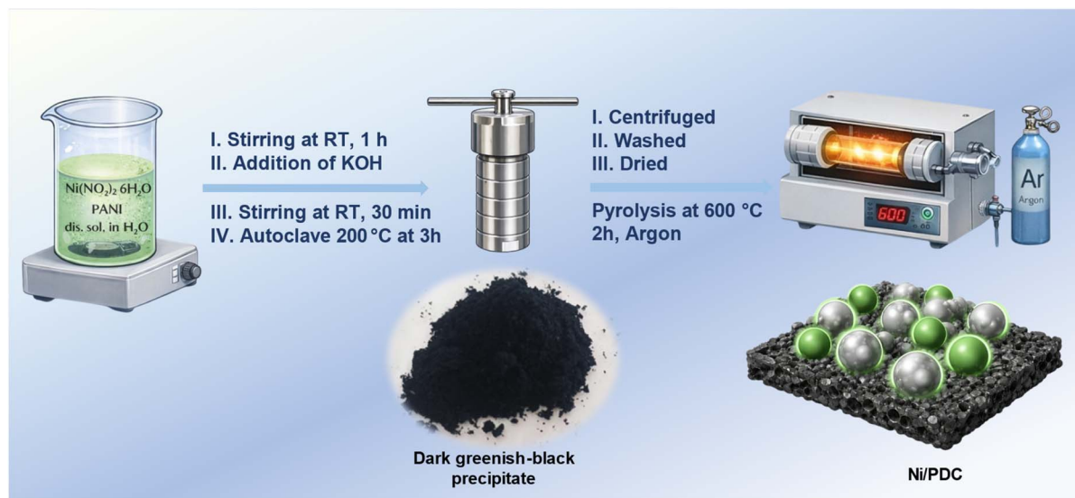
Fig. 1 Ni/PDC catalyst schematic representation.
