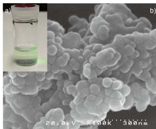
Fig. 8 (a) Laser light scattering of aqueous dispersion of 7. (b) FE-SEM image of spherical organizations made of 7.
