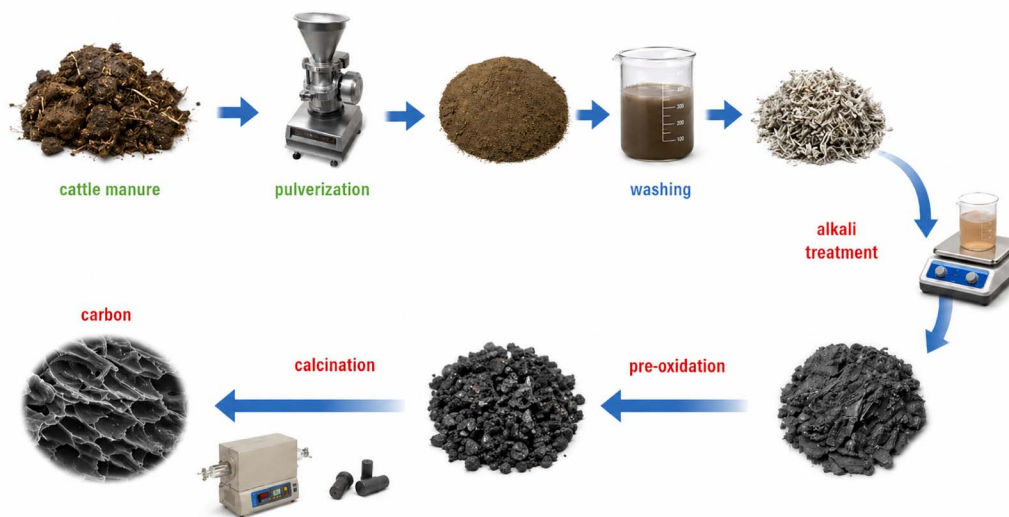
Fig. 1 Schematic illustration of the preparation route for cattle-manure-derived carbon hosts for lithium–sulfur batteries, including water washing, alkali treatment, acid hydrolysis, oxidative stabilization, and carbonization at 650, 850, 1000, or 1050 °C.
