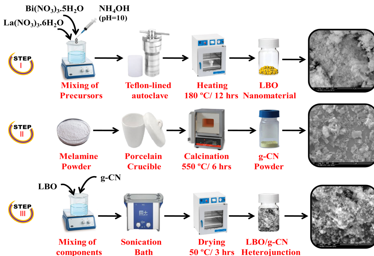
Fig. 1 Schematic presentation of BO, LBO, g-CN, and LBO/g-CN synthesis.
