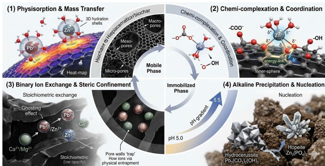
Fig. 12 Schematic illustration of the proposed mechanisms for \text{Pb}^{2+} and \text{Zn}^{2+} immobilization in biochar-amended soil.
