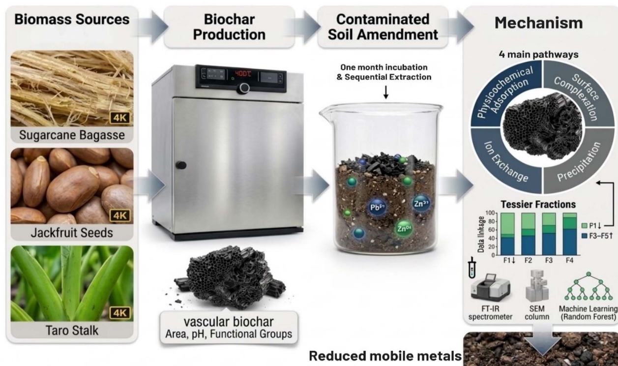
Fig. 1 Schematic illustration of the experimental workflow, including biochar production from different biomass feedstocks, biochar characterization, soil amendment and incubation, sequential extraction of Pb and Zn, and the associated immobilization mechanisms.
