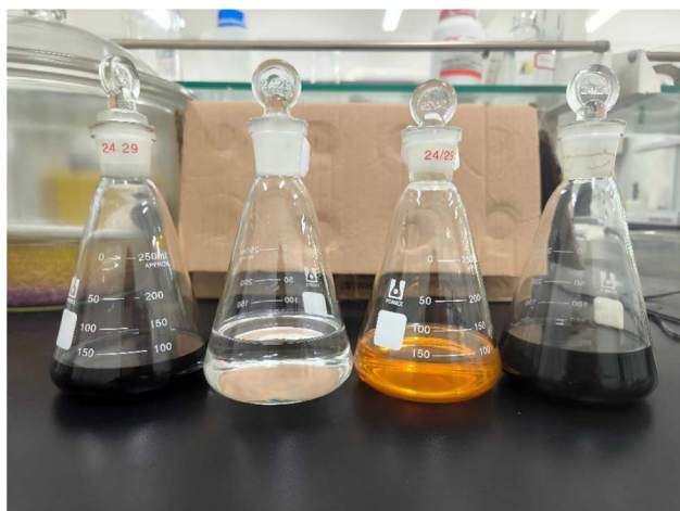
Fig. 7 The four fractions separated by column chromatography elution (the image displays SARA fractions as solutions in their respective extraction/elution solvents prior to rotary evaporation and drying) (from left to right: asphaltene, saturated, aromatic, and resins).
